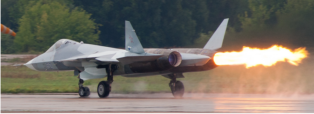
Figure I.2: Compressor stall visualization on a Sukhoi Su-57 prototype, by Rulexip via Wikipedia Commons.
