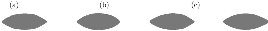
Figure 6.8: (a) Reference optimal shape for the minimum drag test case at Re = 1 with n_p = 5 control points and fixed inner curvature radius. (b) Same as (a) with n_p = 7 control points and fixed inner curvature radius. (c) Same as (a) with n_p = 5 control points and variable inner curvature radius. (d) Reference optimal shape discretized with n_p = 7 control points, after DRL has adjusted the end and inner curvature radii to restore the proper cross-sectional area.
