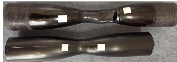
Figure 3.38: Plastic deformation and ductile damage at RH50 for the sample after tension-torsion test in comparison with the initial sample.
