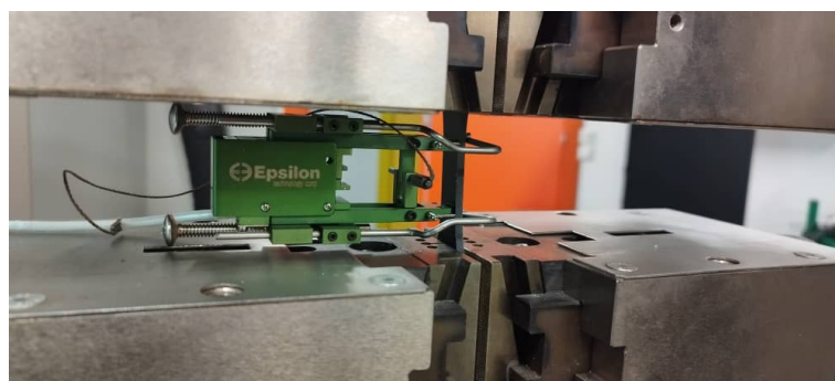
Figure 3.7: Measurement of displacement of dog bone samples using extensometer.
