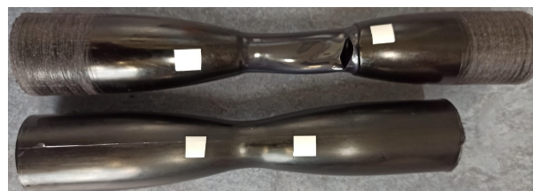
Figure 3.38: Plastic deformation and ductile damage at RH50 for the sample after tension-torsion test in comparison with the initial sample.
