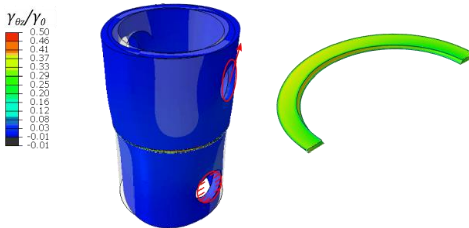
Figure 17: Deformed state of the napkin ring test
