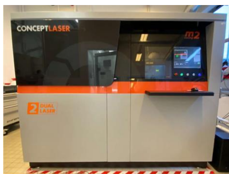
Figure II-4. Installation L-PBF Concept Laser M2 dual laser
