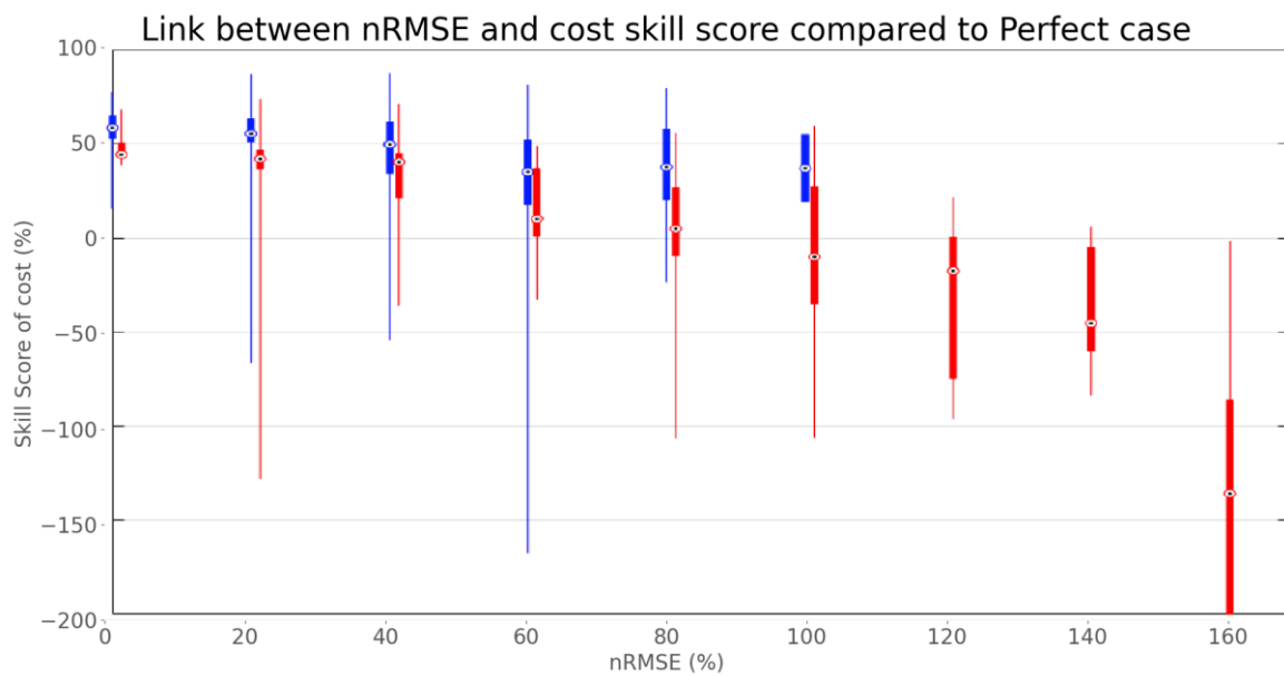
Figure 6.10 Link between nRMSE and daily cost skill score using different forecasts in boxplots
