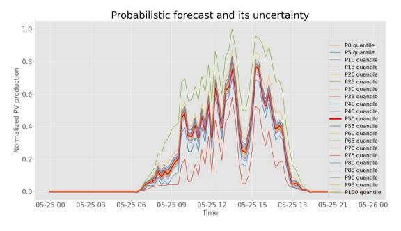
Figure 4.11 Display of probabilistic forecast and its uncertainty range
