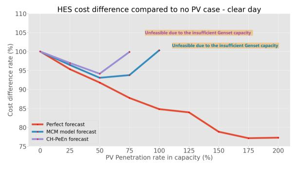
Figure 5.6 Simulation result of clear day situation with P0-P50 and 10% buffer
