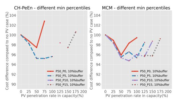
Figure 5.14 Cost difference compared to no PV case with different minimum percentiles at variable situation
