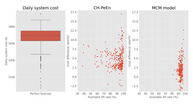
Figure 5.4 Link between risk and cost difference of differents methods compared to Perfect case
