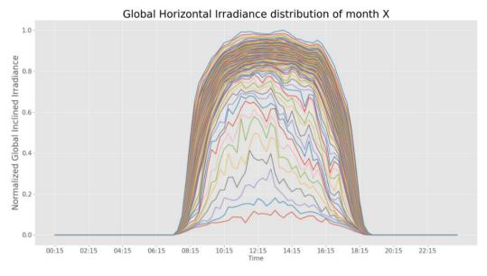
Figure 3.18 Example of a climatological forecast model for January of 10-year combined data
