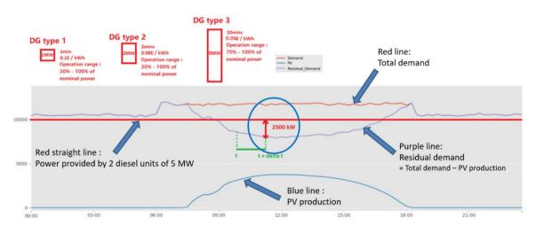
Figure 2.1 Simulation result of a simplified Hybrid Energy System
