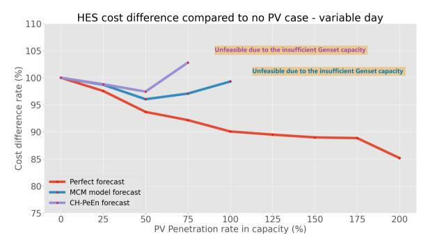
Figure 5.11 Simulation result of variable day situation with PO-P50 and 10% buffer
