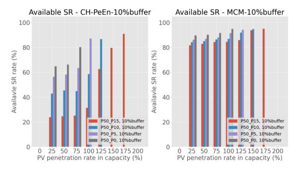
Figure 5.16 HES available SR rate in different minimum percentiles and PV penetration rates
