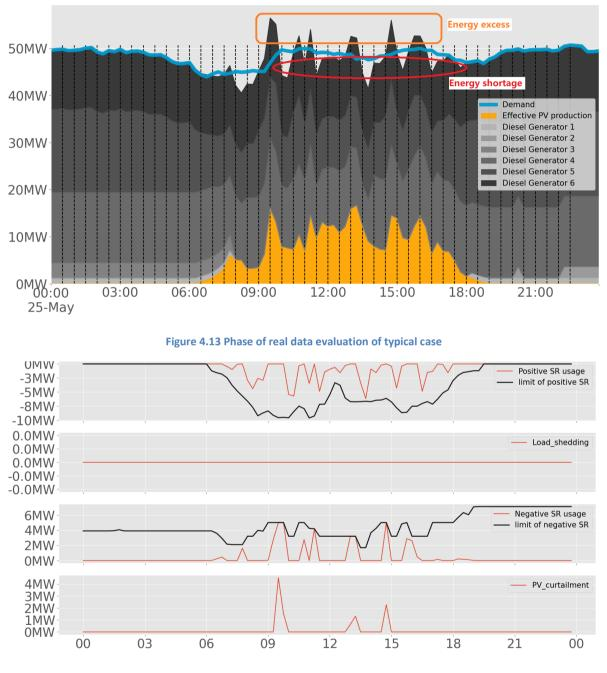
Figure 4.14 Detail of real data evaluation phase of typical case
