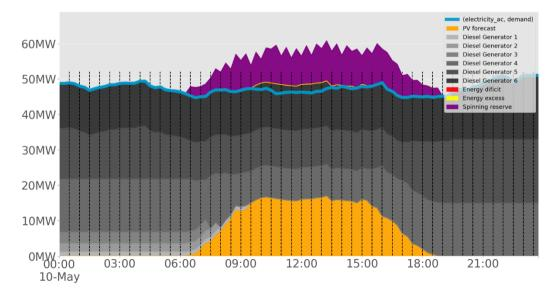
Figure 5.9 Simulation dispatch order with MCM model forecast and 1-hour forecast horizon
