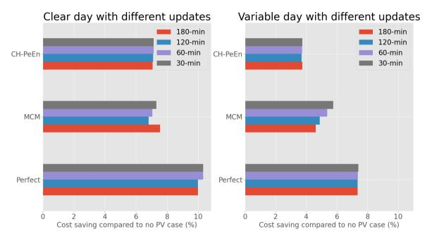
Figure 5.20 Economic cost saving compared to no PV case by using different forecasts with different update times
