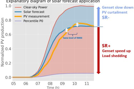
Explanatory diagram of solar forecast application
