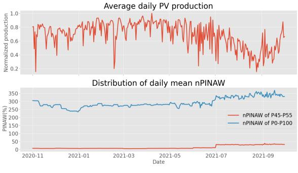
Figure 6.12 Explanation of CH-PeEn PINAW sudden growth
