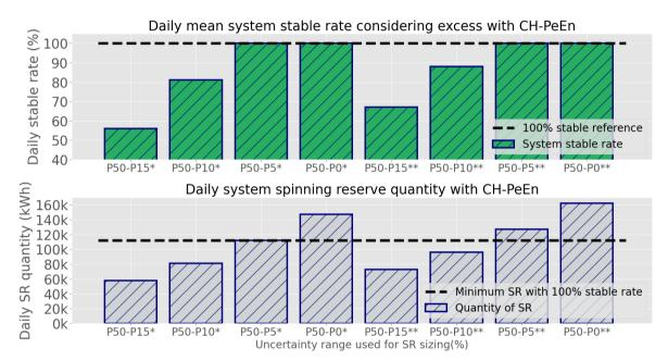
Figure 5.17 System stability and its associated spinning reserve quantity using CH-PeEn forecast with different uncertainties at variable day situation (\* means with extra buffer of 5% PV capacity for SR sizing, \*\* for 10%)
