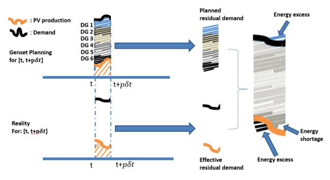
Figure 4.8 Illustration of real data evaluation process in simulation
