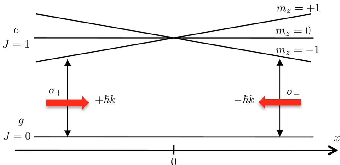
FIGURE 3.7: **Basic principle of the magneto-optical trap (one-dimensional version).** The radiation pressure force created by each light wave depends on the position due to the presence of a magnetic field gradient. The resultant of the two radiation pressure forces is a restoring force towards the origin. The figure is from [71].
