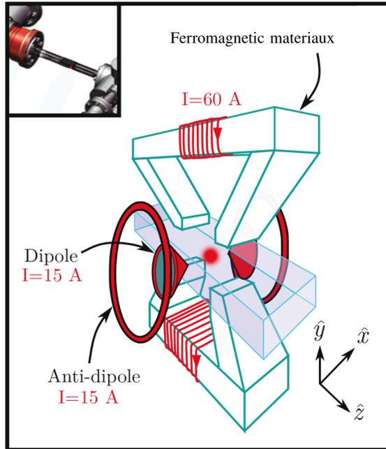
FIGURE 3.9: **Realization of our magnetic trap.** The magnetic trap is formed by combining a quadrupole field generated by an electromagnet of 60 A, and a dipolar field created by a pair of coils of 15 A.
