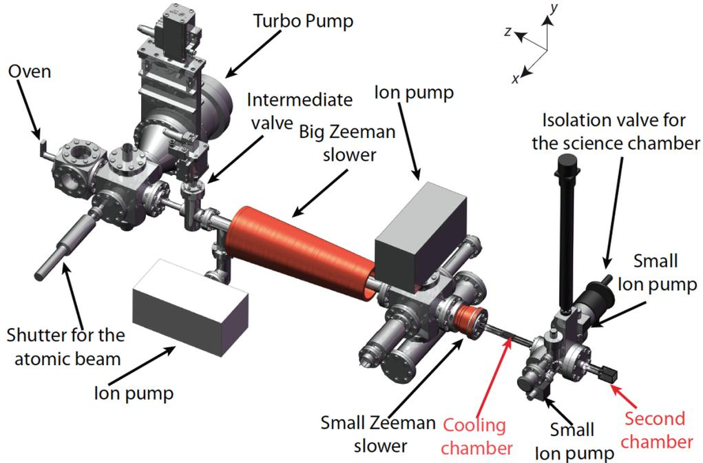
FIGURE 3.4: **Global view of the experimental apparatus.** The axis  $x, y, z$  are set in the way shown in the figure and this standard of the axis will be used in this manuscript and in our experiment.
