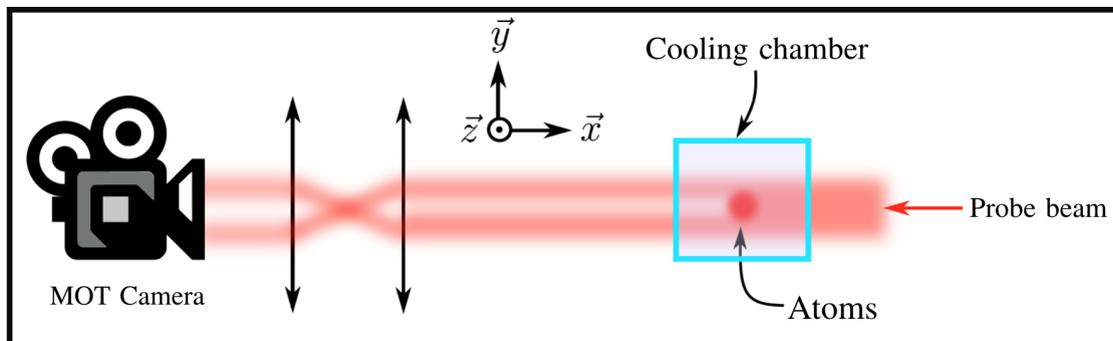
FIGURE 3.18: **Absorption imaging.** A collimated beam is sent to the atoms, which can absorb a part of the photons. So the camera takes an image of the laser with a part of photons absorbed by the atoms and another image of the laser without atoms. By comparing the two images, we can determine the atomic density integrated along the longitudinal direction of the beam. The camera for imaging in the cooling chamber is called 'MOT camera'.
