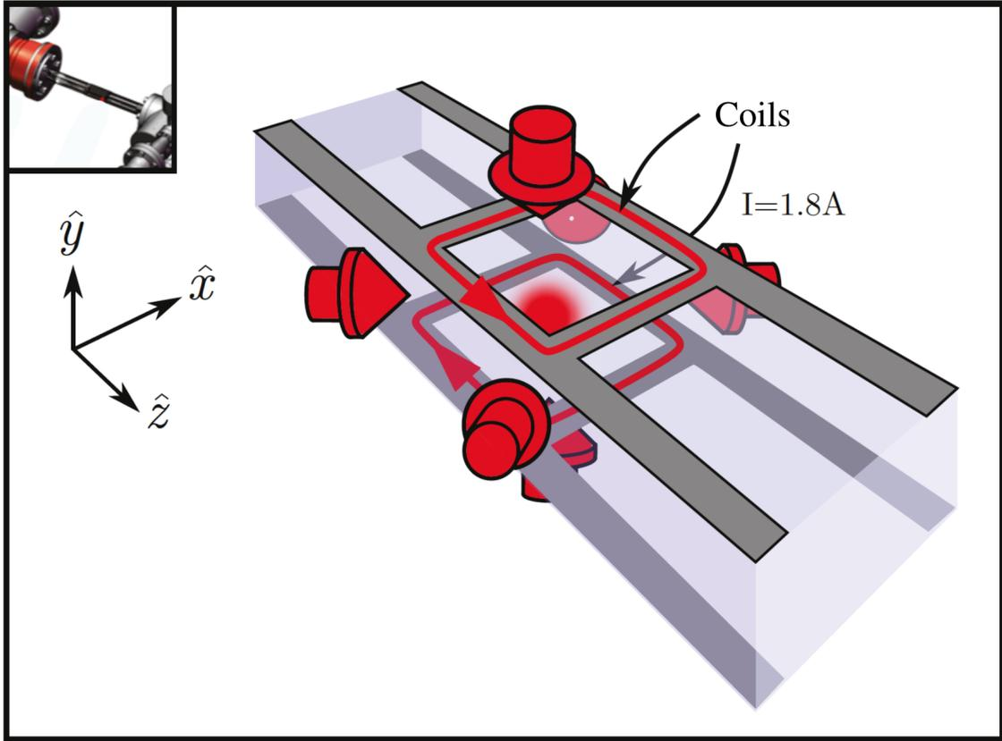
FIGURE 3.8: **Magneto-optical trap in our experiment.** Three pairs of counter-propagating lasers and a magnetic gradient can cool and trap the atoms (magneto-optical trap). The three pairs of lasers come from the *cluster*, and each laser is about 15mW.
