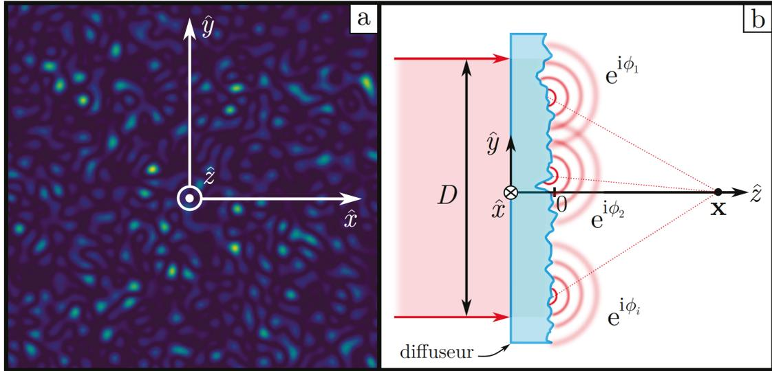
FIGURE 4.1: **Speckle field and its generation.** **a**, The speckle field consists of a random distribution of light intensity. **b**, The diffuser prints a random phase to the wavefront.
