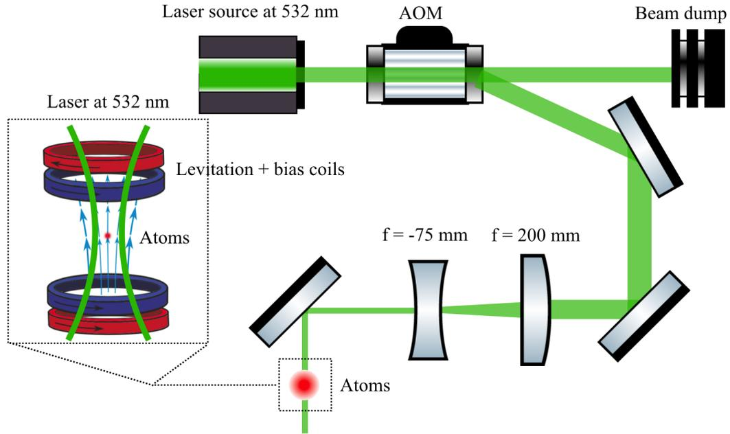
FIGURE 7.11: **Set-up of the anti-trap.** The laser comes from a source of high-power laser of 532 nm. The beam waist is about 1.125 mm. It is diffracted by an AOM, and the order 0 is shone into a beam dump for security. Then beam is shaped to have a small waist of about  $420 \mu\text{m}$  by a telescope, and goes to the atoms. Near the atoms, the beam is along the y-axis (vertical direction), therefore the anti-trap is for the x- and z-axis.
