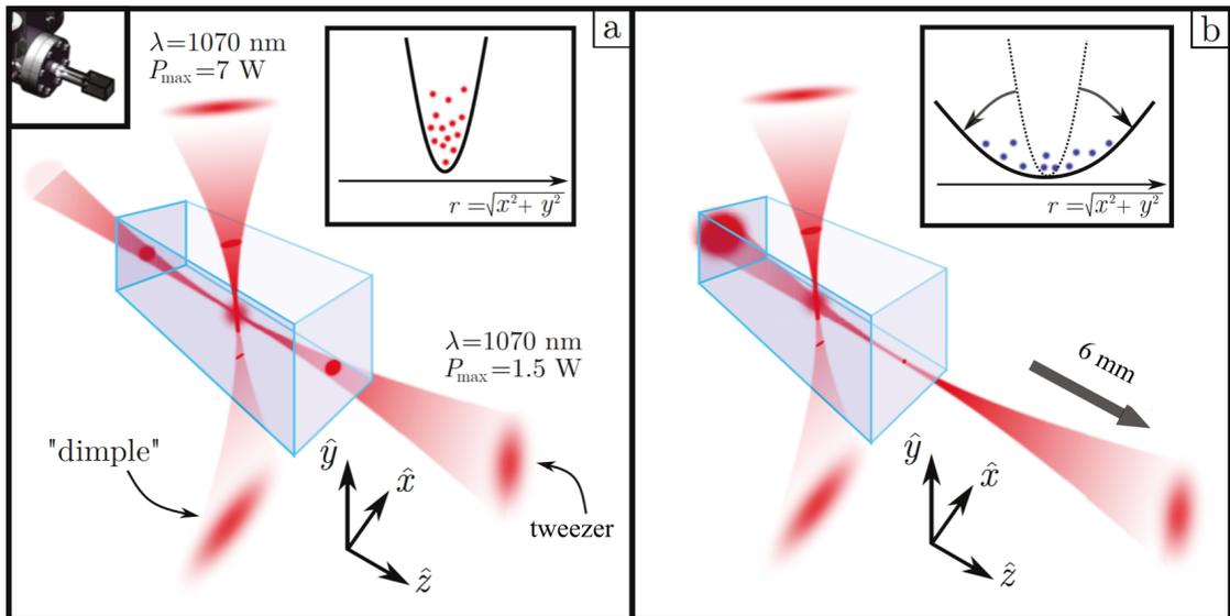
FIGURE 3.13: **Crossed optical dipole trap and adiabatic opening.** **a**, the configuration of the crossed optical dipole trap. **b**, the adiabatic cooling through moving the focus of the tweezer beam by 6 mm along  $z$  direction.
