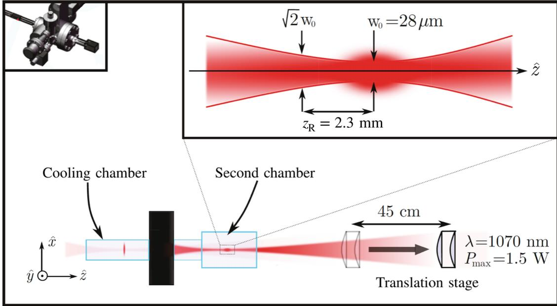
FIGURE 3.11: **Optical tweezer and translation of the atoms.** The laser beam is focused to the atoms by a lens to have a waist of  $28 \mu\text{m}$ . The lens is mounted on a translation stage. The atoms trapped by the focal point of the laser are translated by 45 cm from the cooling chamber to the second chamber.
