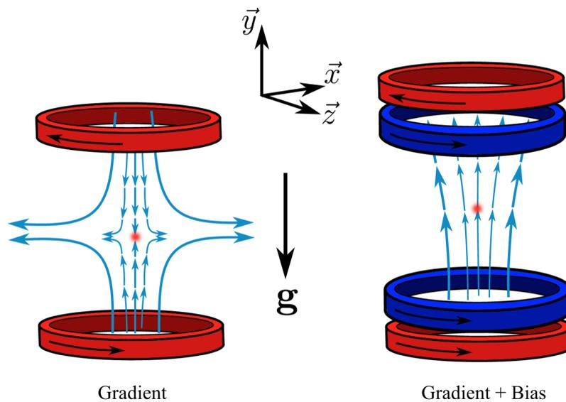
FIGURE 3.15: **The coils for the magnetic levitation.** The coils in the anti-Helmholtz configuration generate the magnetic gradient field (red coils). The coils in the Helmholtz configuration generate the magnetic bias field (blue coils). On the right, the magnetic field is the situation for a strong bias field.
