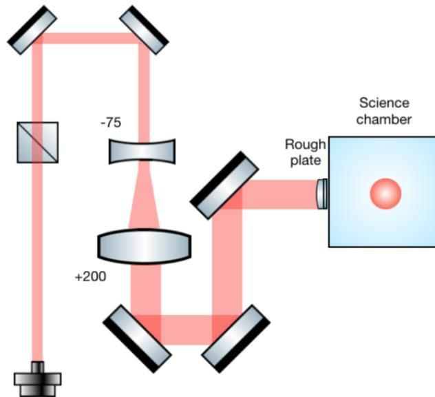
FIGURE 4.5: **Experimental realization of speckle beam.** At the output the fiber, the waist of the beam is 5.6 mm. The beam waist is then broadened to 14.6 mm by a telescope before going to the science chamber.
