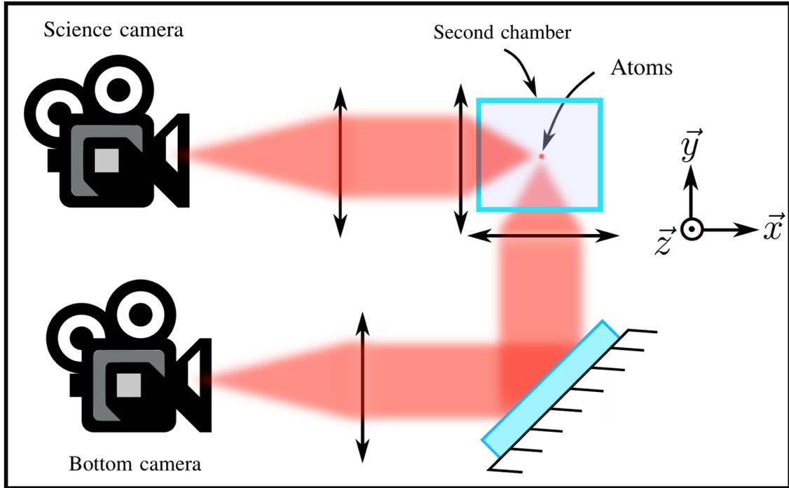
FIGURE 3.19: **Fluorescence imaging.** The beam for fluorescence imaging is about 10 mW. We have two cameras to perform a 3D imaging.
