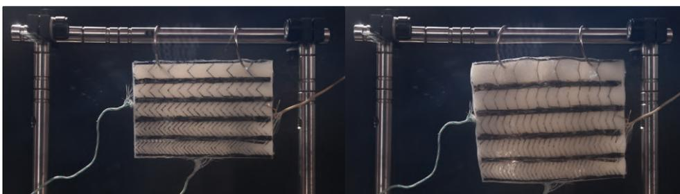
Figure 2.12 Samples with parallel lines linked with chevrons at room temperature (left) and at 90°C (right).
