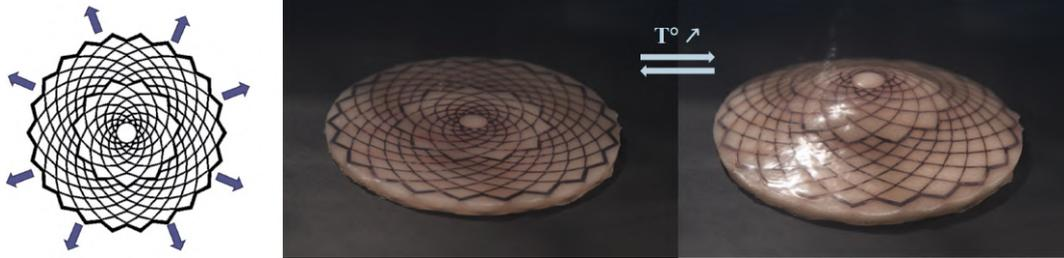
Figure 2.44 Diamonds network made with logarithmic spirals. For all the diamonds, the ratio  $C_i < 1$ . The diamonds are thus elongated along the perimeters and grow radially. When the matrix expands, a conical shape emerges.
