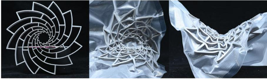
Figure 3.48 Logarithmic spirals with an angle  $\beta = \frac{\pi}{3}$ . The aspect ratio of the cells  $\frac{l}{d}$  as well as the ratio  $\frac{e}{l}$  are kept constant. As the cells close, a shape with a negative Gaussian curvature emerges.
