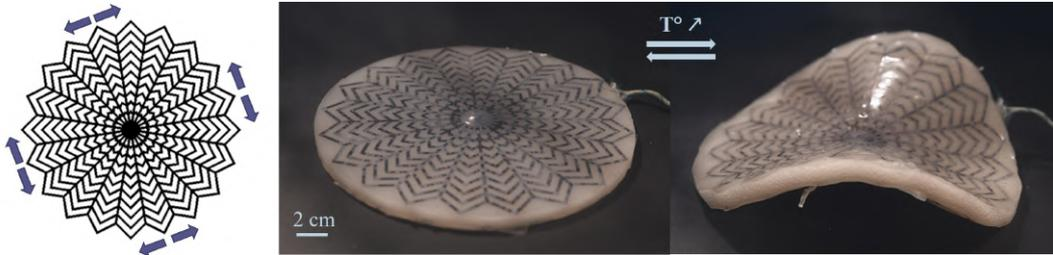
Figure 2.29 Network of chevrons with radial thick lines. When the temperature is increased, a shape of an e-cone emerges and goes back to the flat state when the temperature is lowered. On the left the Mylar network before being embedded in the matrix.
