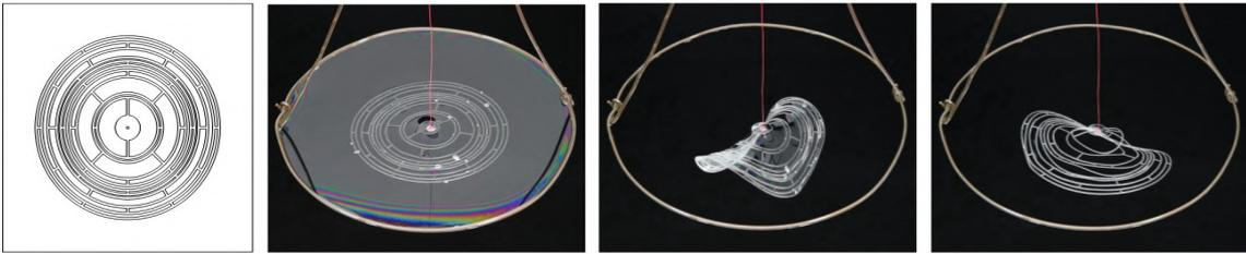
Figure 4.21 Network with orthoradial cells with soap film. From left to right: the design, the shape before and after being deformed by the soap and the shape when all the soap films have disappeared.
