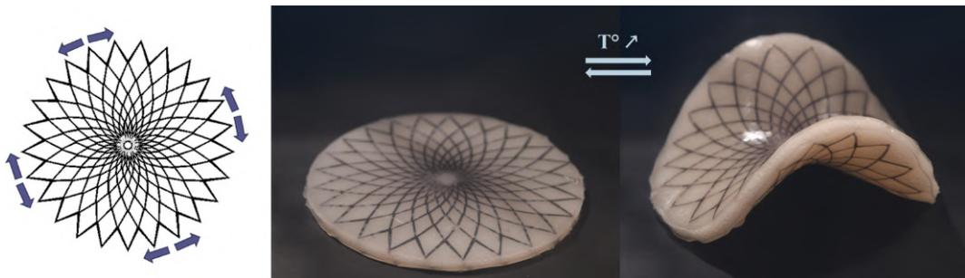
Figure 2.45 Diamond networks made of logarithmic spirals. For all the diamonds, the ratio  $C_i > 1$ . The diamonds are elongated along the radii and grow azimuthally. When the matrix expands, a saddle shape emerges.
