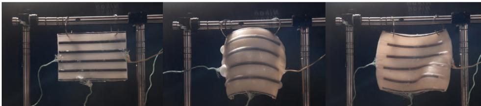
Figure 2.11 Sample with parallel lines at room temperature (left) and 90°C (center and right). The two samples (center and right) behave differently but do not remain in plane.
