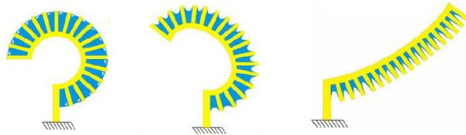
Figure 4.1 Fern capsule model opened with capillary forces [116] [113]
