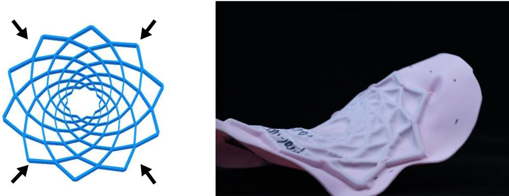
Figure 3.42 Diamond network organized along logarithmic spirals with small angle  $\theta > \frac{\pi}{4}$ . When the sample is put under vacuum, the cells close in the radial direction and an e-cone emerges
