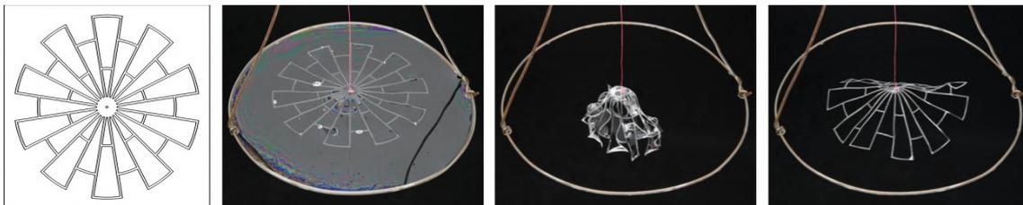
Figure 4.18 Network with radially elongated cells shrunk by soap films. On the left, the design then the network before, after being deformed by the soaps films, and finally the shape when all soap films burst.
