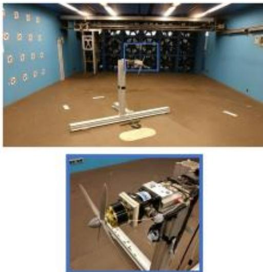
**Fig. 3** Isolated small-scale propeller mounted in the L2 subsonic wind tunnel
