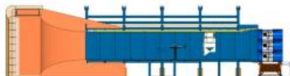
**Fig. 4** Scheme of the INTRON bench mounted in the L2 subsonic wind tunnel
