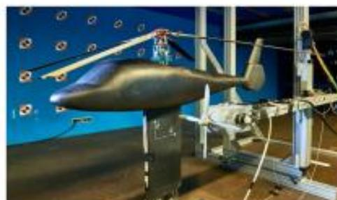
Fig. 2 Installation of the full assembly in the L2 wind tunnel
