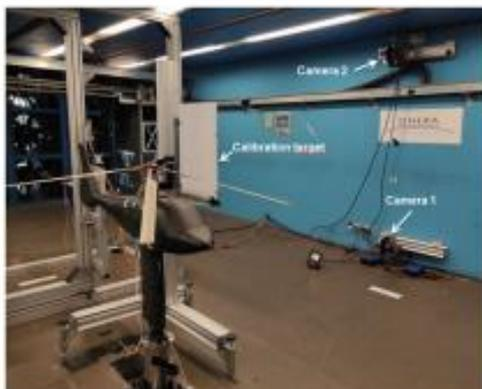
**Fig. 7** Implementation of the PIV setup in the L2 wind tunnel during calibration
