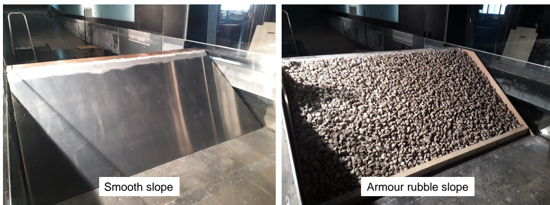
Figure 5.4: Photograph of the breakwater with smooth (left) and armoured rubble (right) slopes.
