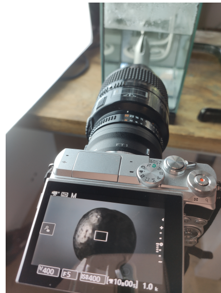
(c) Picture of the sphere from the camera viewpoint. The focus was set to have the sphere on the plane of sharpness.
