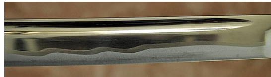
Figure 1.2: Double quenched katana with “Hamon Notare” finition (from Géry PAR-ENT).
