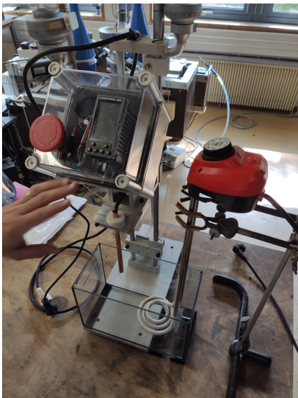
(b) Picture of the quenching bath. The immersed heater is on the right of the bath. The thermocouple is not shown here, but was placed opposite to the heater. The rod is the set up of another ongoing experiment.
