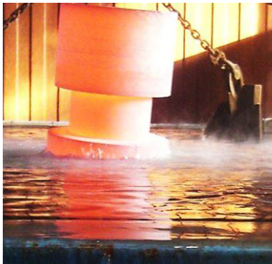
(a) Industrial quench of a hollow cylinder. (b) Industrial quench of a metallic spring.
