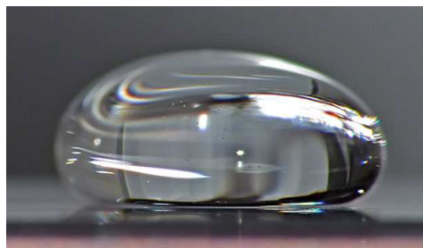
(d) Calefaction under a water drop over a heater (from [19])
