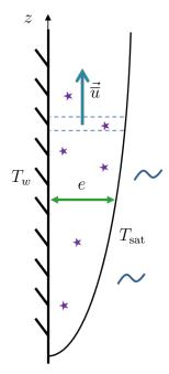
(a) Description of the Boundary Layer vapour film. Buoyancy effects make the vapour rise. It is limited by internal viscous forces. The layer thickness increases as vaporisation feeds the vapour film.
