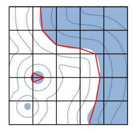
(a) Volume Of Fluid method. A volume fraction function identifies one phase from another. The interface can be reconstructed providing a sufficient mesh precision.
