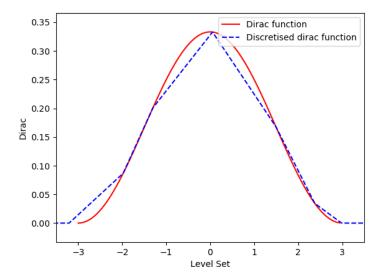
Figure 3.12: Example of discretisation of the Dirac function  $\delta_{\alpha}$  in 1D. A thousand similar discretisations are done in the same way using randomised positions around the reference points.
