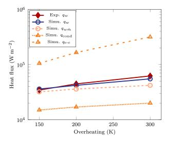
Figure 6.21: Comparison of experimental [57] and simulated wall heat fluxes of the saturated vertical film boiling case. Orders of magnitude and trends are respected between the simulation and the experiments. The evaluation from the mass flux leads to a moderate mass loss at high overheating. The conductive estimation understimates a lot the heat flux, as it does not take into account the wetting model, whereas the conductive-convective overestimates a lot the heat flux.
