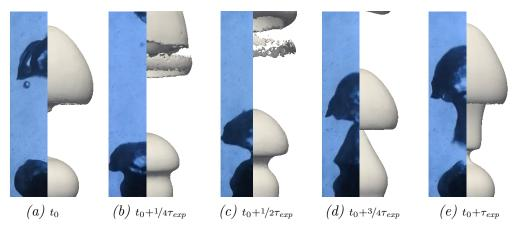
Figure 5.17: Comparison of experimental bubble profile with the simulation for  $T_S = 800 \,^{\circ}\text{C}$ ,  $T_{\infty} = 98 \,^{\circ}\text{C}$ .
