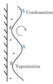
(a) Description of the vaporization—condensation cycle. The liquid vaporise in the valleys of the wave, where heat fluxes inside the vapour are very intense. Vapour condenses at the top of the bulges where vapour heat fluxes are moderate.
