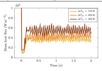
Figure 6.20: Wall heat flux over time for the saturated vertical film boiling simulation at different overheating. 1s is shown to be enough for the hydrodynamic steady state to be reached.
