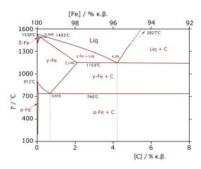
Figure 1.3: Iron Carbon phase diagram. At high temperature and low carbon concentration, the austenite phase is stable. However, if this phase is cooled down slowly, it turns into perlite. The desired martensite phase is not on this graph as it is not a thermodynamical optimum (from MARKEL-LOS).
