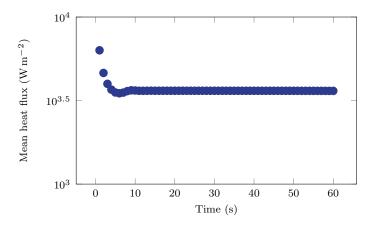
Figure 6.24: Wall heat flux over time for the natural convection simulation. The final time considered it large enough to quaranty the steady state regime.
