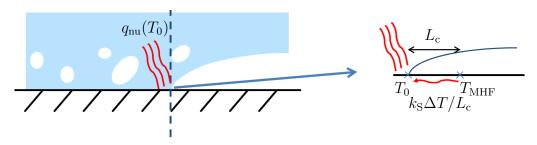
Figure D.6: Schematic description of wetting front. The intense heat flux at the wetting front (for  $T = T_0$ ) is compensate by a diffusive heat flux at the surface of the plate. Thus the "macroscopic" wetting temperature is larger.
