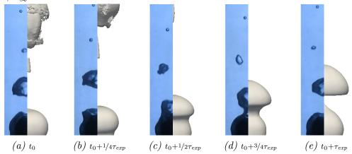
Figure 5.18: Comparison of experimental bubble profile with the simulation for  $T_S = 600 \,^{\circ}\text{C}$ ,  $T_{\infty} = 95 \,^{\circ}\text{C}$ .
