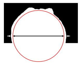
Figure 5.6: Measurement of the vapour film thickness. The length of the line of white pixels at the height of the sphere equator is measured. This corresponds to the sum of the diameter of the sphere and of two vapour film thicknesses.
