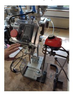
(b) Picture of the quenching bath. The immersed heater is on the rigth of the bath. The thermocouple is not shown here, but was placed oposit to the heater. The rod is the set up of another ongoing experiment.
