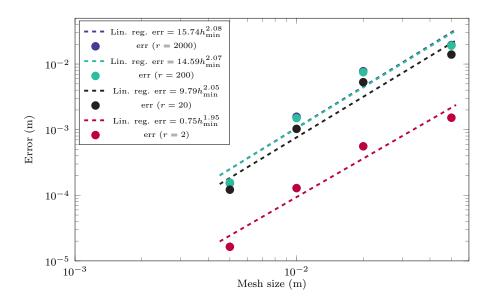
Figure 3.10: Space-time convergence analysis for the Moving Interface benchmark for  $\varepsilon = 0.1 \,\mathrm{m}$ .
