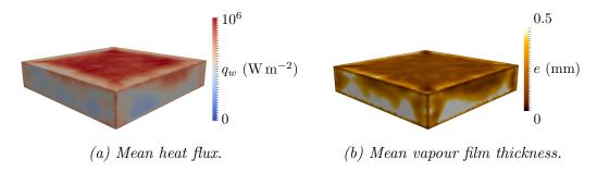
Figure 7.7: Visualisation of the simulated mean solid heat flux and vapour film thickness for the brick quenching simulation. Heat fluxes are more intense at the top of the brick and at the edges where the vapour film is the thinnest.
