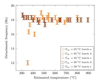
Figure 5.14: Experimental measurements of the vapour bubbles detachment frequency from the sphere for liquid temperatures of  $T_{\infty} = 95$  °C and  $T_{\infty} = 98$  °C.
