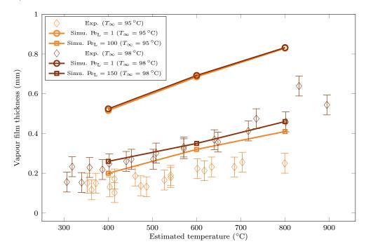
Figure 5.20: Comparison of experimental and simulated vapour film thicknesses at the equator of the sphere for liquid temperatures of  $T_{\infty} = 95$  °C and  $T_{\infty} = 98$  °C.
