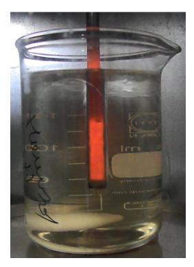
Figure 7.10: Picture of the drasticity test at one second after the start. The vapour film is very flat and regular around the rod.
