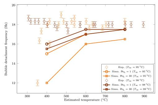
Figure 5.22: Comparison of experimental and simulated vapour bubble detachment frequency for liquid temperatures of  $T_{\infty}=95\,^{\circ}\mathrm{C}$  and  $T_{\infty}=98\,^{\circ}\mathrm{C}$ .
