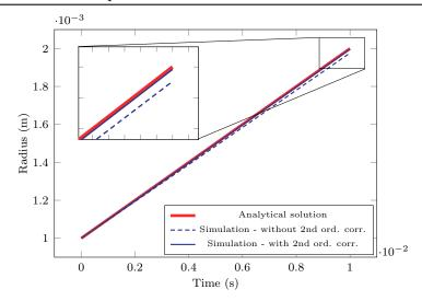
Figure 3.15: Impact of the 2nd order correction term on the LS convection velocity the Growing Bubble benchmark for  $\varepsilon = 2 \times 10^{-4} \,\mathrm{m}$ .
