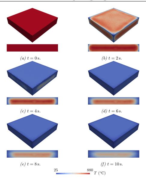
Figure 7.8: Top and cross section views of the temperature field from the thermal simulation of the brick quenching case for different time steps. The edges are the areas where the brick is cooled the fastest, in opposition to the center.
