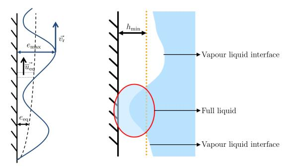
Figure 6.15: The equivalent Boundary Layer profile.  $e_{eq}$  and  $\overline{u}_{eq}$  are targeted to conserve the mass flux.
