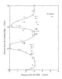
(b) Magnitude of the normal velocity component of liquid particles. This highlights the recirculation effects at play at the interface.
