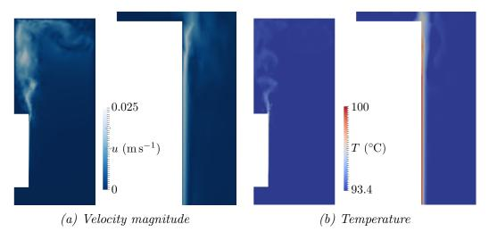
Figure 6.23: Final velocity temperature fields of the monophasic natural convection simulation.
