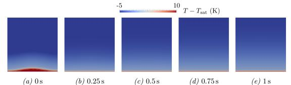
Figure 4.25: Phase distribution and temperature of the 2D computation of the 5K horizontal film boiling with 1K subcooling.
