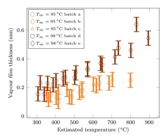
Figure 5.12: Experimental measurements of vapour film thicknesses at the equator of the sphere for liquid temperatures of  $T_{\infty} = 95$  °C and  $T_{\infty} = 98$  °C.
