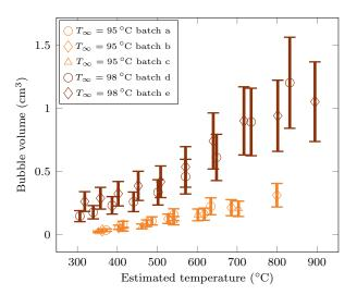
Figure 5.13: Experimental measurements of vapour bubble volumes for liquid temperatures of  $T_{\infty} = 95$  °C and  $T_{\infty} = 98$  °C.
