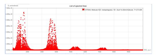
Figure A.2: The spectral line strength S profile is computed for water vapour at  $1000\,^{\circ}$ C (credits: simulation from Hitran [146])
