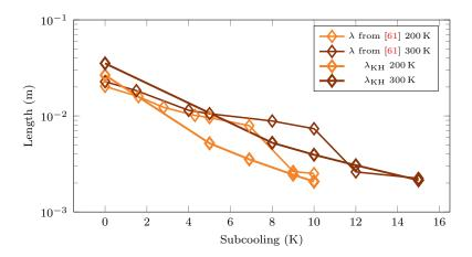
Figure 6.7: Comparision of experimental wavelengths  $\lambda$  [61] with the most dangerous wavelengths  $\lambda_{KH}$  in regards to the Kelvin–Helmholtz instability theories of [139].
