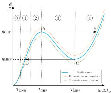
Figure 1.8: The boiling curve. The liquid is supersaturated 0 before the Onset of Nucleate Boiling. Nucleate boiling starts with partial 1 and fully developed 2 mode until it reaches the Critical Heat Flux (point A). Then the heat flux decreases during transition boiling 3 to reach the Minimum Heat Flux (point C). Then calefaction 4 starts and the heat flux increases slowly until radiation takes the lead at very high temperatures.
