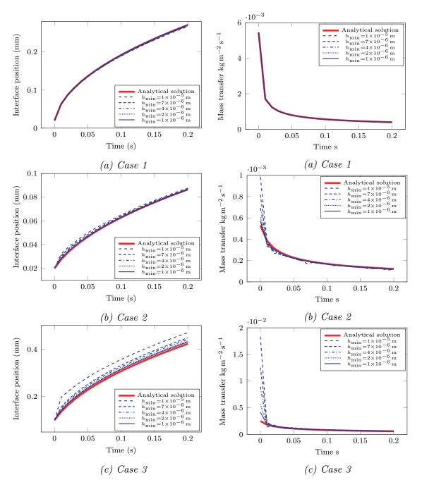
Figure 2.14: Analytic and simulated posi- Figure 2.15: Analytic and simulated mass tions of the interface for different mesh sizes transfer rates for different mesh sizes h.
