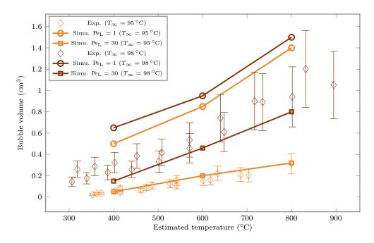
Figure 5.21: Comparison of experimental and simulated vapour bubble volumes for liquid temperatures of  $T_{\infty} = 95$  °C and  $T_{\infty} = 98$  °C.
