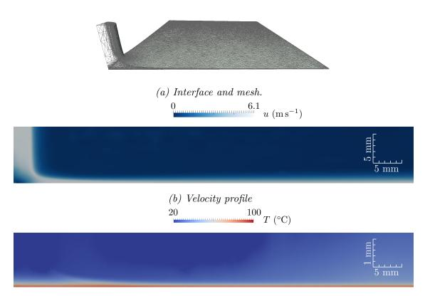
(c) Temperature profile close at the bottom. The z dimension has been streched by a factor 5 to better see the temperature gradients.
