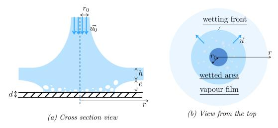
Figure D.1: Global description of the water jet quenching process.
