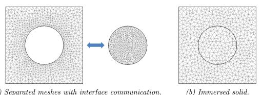
(a) Separated meshes with interface communication.
