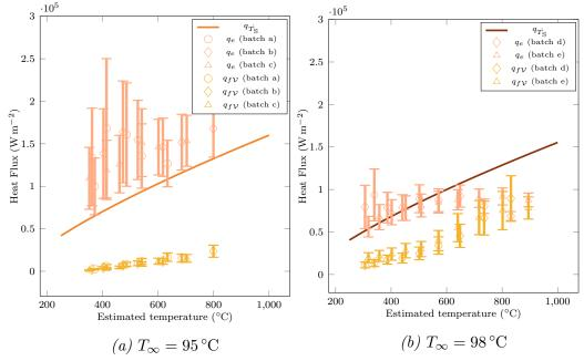
Figure 5.15: Comparison of experimental heat fluxes from the cooling rate estimation  $q_{\hat{T}_S}$ , the vapour film thickness  $q_e$  and the vaporisation  $q_{f\mathcal{V}}$ .  $q_e$  overestimates the heat fluxes for  $T_{\infty} = 95\,^{\circ}\mathrm{C}$  and at lower overheating for  $T_{\infty} = 98\,^{\circ}\mathrm{C}$ . The energy budget to vaporise the liquid  $q_{f\mathcal{V}}$  is negligible for the  $T_{\infty} = 95\,^{\circ}\mathrm{C}$ .
