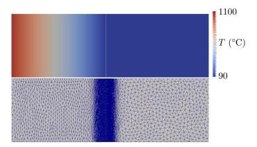
Figure 2.12: Temperature field and mesh of the Case 3 simulation for  $h = 2 \times 10^{-6}$  m at time 0.1 s. The mesh is refined around the interface where temperature gradients and physical properties variations are important. Only the left side of the computational domain is plotted.
