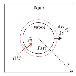
Figure C.1: Representation of Growing Bubble case.
