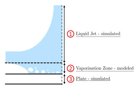
Figure D.5: Separation of the problem of Jet Quenching. The liquid zone  $\bigcirc$  and the solide zone  $\bigcirc$  were simulated. The vaporisation zone  $\bigcirc$  was modeled.
