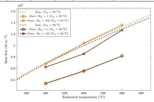
Figure 5.23: Comparison of experimental and simulated heat fluxes for liquid temperatures of  $T_{\infty} = 95$  °C and  $T_{\infty} = 98$  °C.
