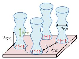
(b) Vapour jets of fully developed boiling. The CHF is reached when  $u_{KH}$  and thus  $d_{KH}$  are so large that the liquid can't replace the vapour at the bottom of the jets.
