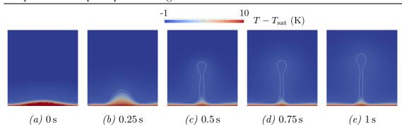
Figure 4.22: Phase distribution and temperature of the 2D computation of the 1K horizontal film boiling with 1K subcooling.
