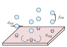
(a) Partial nucleate boiling. Bubbles of diameter  $d_{NB}$  leave the nucleation sites of density  $N_{NB}$  at a frequency  $f_{NB}$ .
