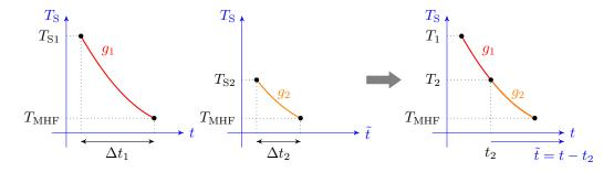
Figure 5.3: Graphical view of the master cooling curve. If the cooling rate is only a function of the temperature, then the two cooling curves of two different initial temperatures overlap on the same master curve.
