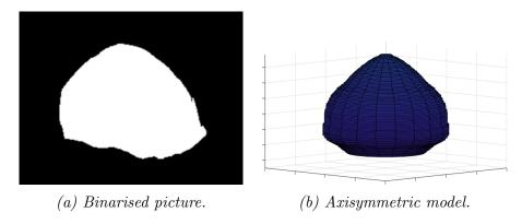
Figure 5.7: Axisymmetric 3D model of a vapour bubble recovered from a 2D binarised picture. The length of each line of white pixel is considered to be an infinitesimal cylinder. The sum of these cylinder represents an estimation of the bubble volume.
