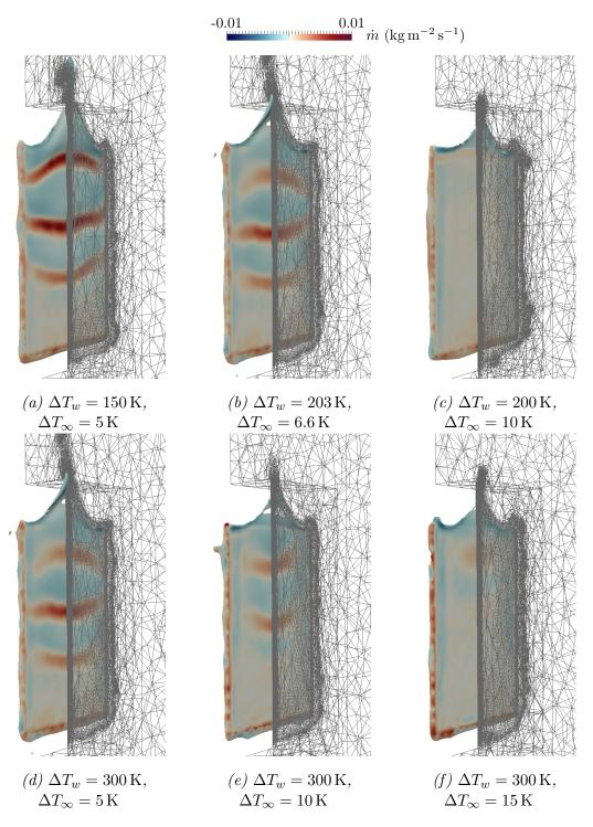
Figure 6.26: Visualisation of the liquid vapour interface at the last increment (t = 2s) of the subcooled vertical film boiling simulation for different overheatings and subcoolings.
