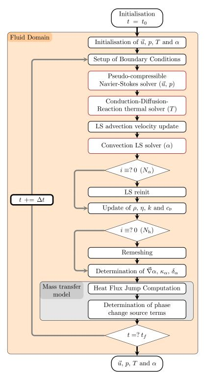
Figure 4.1: Solving procedure of the phase change solver.
