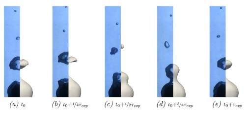
Figure 5.27: Comparison of experimental bubble profile with the simulation for  $T_S = 600\,^{\circ}\text{C}$ ,  $T_{\infty} = 95\,^{\circ}\text{C}$  with the convective conductivity model for  $Pe_L = 30$ .
