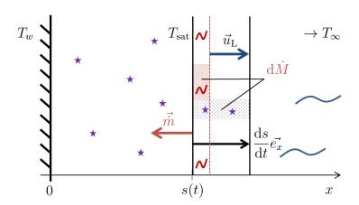
Figure 4.4: Description of the compressible Stefan problem. The wall to the left is at  $T_w$ , and the liquid to the right is at  $T_\infty$  far from the interface. The heat flux from the wall gives energy to the interface by conduction. The liquid heats up and vaporises, but conduction in the liquid slows down the interface progress. As the liquid is more dense, its vaporisation creates a volume. The vapour is blocked by the wall and pushes the liquid back.
