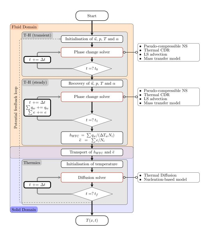
Figure 7.3: Solving procedure of the quenching framework.
