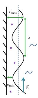
(b) General description of the vertical film waves. Waves are assumed to be periodic with a wavelength  $\lambda$  and a phase velocity  $\vec{v_r}$ . Zones of minimum amplitudes  $e_{min}$  are the "valleys" and areas of maximum amplitude  $e_{max}$  are the peaks.
