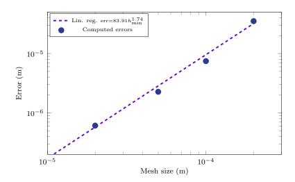
Figure 3.16: Space-time convergence analysis for the Growing Bubble benchmark for  $\varepsilon = 2 \times 10^{-4} \,\mathrm{m}$ .
