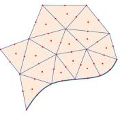
(c) Finite Element Method. Quantities are integrated in Interpolation functions are used to discretise the quantities over the cells (here order 2 polynomials).
