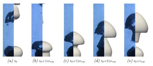
Figure 5.26: Comparison of experimental bubble profile with the simulation for  $T_S = 800$  °C,  $T_{\infty} = 98$  °C with the convective conductivity model for  $Pe_L = 30$ .
