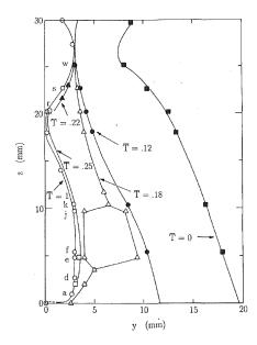
Figure 6.14: Isotherms extracted from [57] for  $\Delta T_w = 160 \,\mathrm{K}$  and  $\Delta T_\infty = 1.6 \,\mathrm{K}$ . Thermal layers are very tiny that lead to intense heat fluxes.
