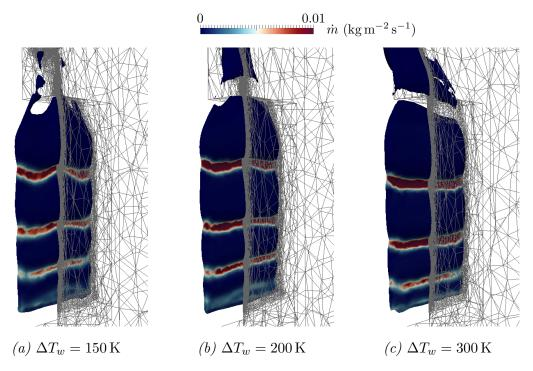
Figure 6.18: Visualisation of the liquid vapour interface at the last increment (t = 2s) of the saturated vertical film boiling simulation for different overheatings.
