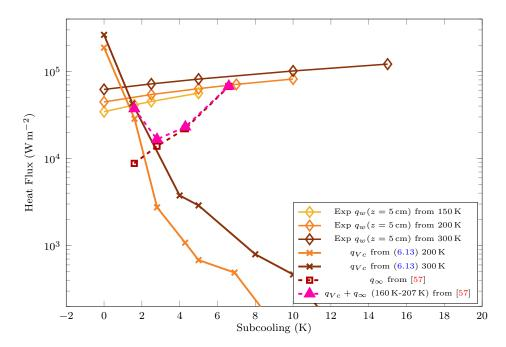
Figure 6.12: Estimation of the energy distribution. A portion of the heat flux should vaporise the liquid  $(q_{Vc})$  while the other part should be used to warm up the liquid  $(q_{\infty})$ . The addition of these two terms should balance measured heat fluxes, which is roughly the case.
