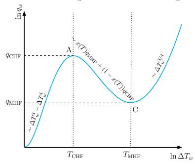
Figure 1.16: Tendancies of the boiling curve from correlations of the literature. The CHF (point A) can be assessed by Zuber's theory, and the MHF (point C) can be assessed by Berenson's theory.
