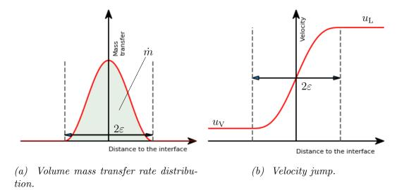
Figure 3.7: Interfacial velocity and mass transfer profiles in the context of smoothed interface and Continuous Surface Force approach.
