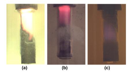
Figure 1.10: Pictures of vapour film fronts from Inconel probe quenched in (a) water, (b) aqueous polymer solution and (c) mineral oil (from [9]).
