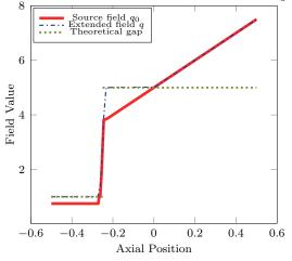
(c) Source and extended field values on the vertical axis x = -0.25
