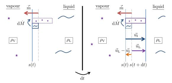
Figure 3.1: Representation of the velocity jump due to the density difference. In this graphic, the vapour phase is static. The extension of the fluid particle that vaporises pushes the liuqid back at a lower velocity than the interface.
