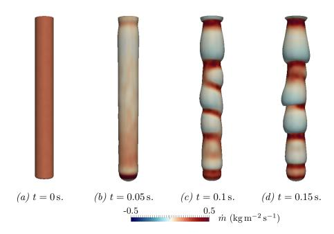
Figure 7.12: Visualisation of the simulated liquid vapour interface and mass transfer rate for the drasticity simulation. The vapour waves are important with vapour created from the bottom and rising along the rod. However this not consistent with experimental observations, as the film should be flatter.
