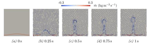
Figure 4.23: Mass transfer and velocity trajectories of the 2D computation of the 1 K horizontal film boiling with 1 K subcooling.
