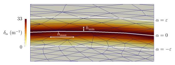
Figure 4.3: Visualisation of the mesh at the interface. The mesh size normal to the interface is correctly set to  $h_{min}$ , while the other dimension is set to  $h_{max}$ . The dirac function is also plotted, for the case  $\varepsilon = 0.3 \,\mathrm{m}$ .
