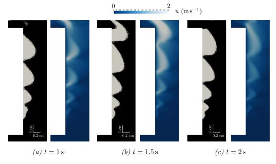
Figure 6.19: Visualisation of a cross section view of the vapour film and of the velocity magnitude for the saturated vertical film boiling simulation with  $T_w = 200\,\mathrm{K}$  at different time steps. The figures are stretched to highlight the waves.
