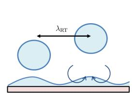
(a) Horizontal film boiling. Vapour bubbles are spaced from each other by the most unstable wavelength of the Rayleigh-Taylor instability theory. The liquid vaporise from the thin parts of the film to feed the bubbles.
