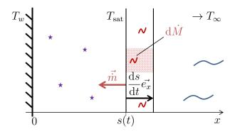
Figure 2.11: Description of the Stefan problem. The wall to the left is at  $T_w$ , and the liquid to the right is at  $T_\infty$  far from the interface. The heat flux from the wall provides heat to the interface by conduction. The liquid heats up and vaporises, but conduction in the liquid slows down the interface progress. As both phases have the same density, the mass transfer does not create any movement in the fluid.
