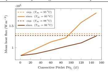
Figure 5.24: Study of the influence of  $Pe_L$  on the vapour heat flux for  $T_{\infty} = 95$  °C and  $T_{\infty} = 98$  °C.
