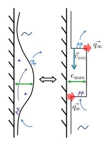
(b) Model of the vaporization—condensation cycle on a bulge. It is assumed that all the fluid particles vaporise and condensate in the vertical direction.
