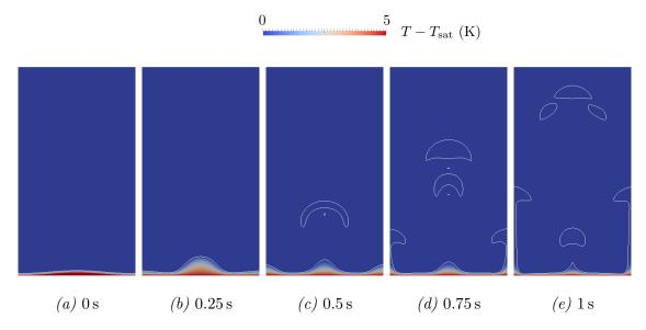
Figure 4.19: Cross section view of the temperature field of the 3D computation of the 5K horizontal film boiling.
