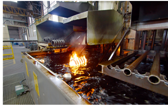
(a) Industrial quench of a hollow cylinder. (b) Industrial quench of a metallic spring.
