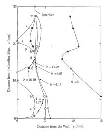
(a) Velocity trajectories in the liquid phase. Recirculations in the liquid are similar to those of a float on a free surface.
