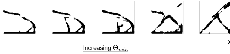
Figure 5.23: Particular geometries generated by a DL model trained to control the \Theta_{min} along the mechanical constraints.
