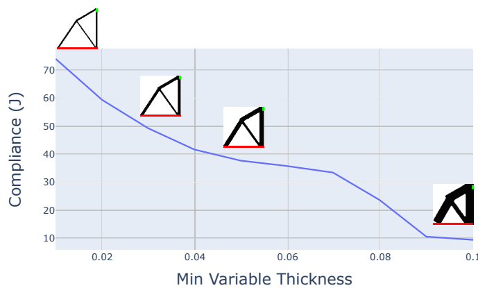
(c) Compliance versus minimum variable thickness.
