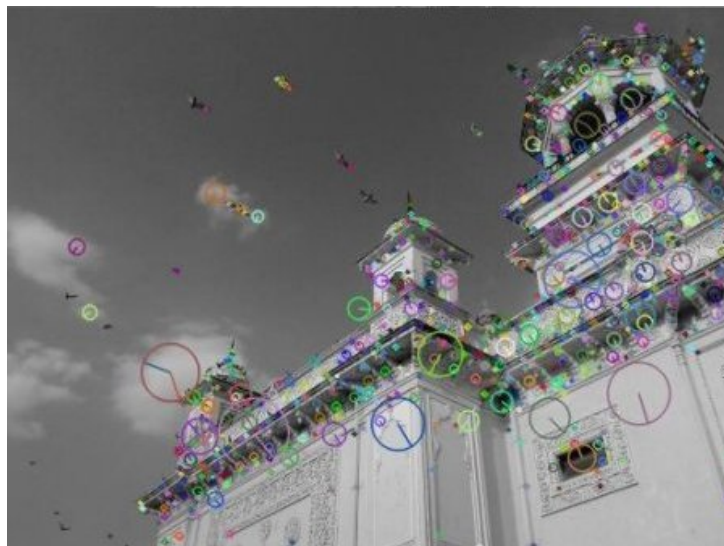
Figure 3.19: SIFT algorithm: example of image key points 8
