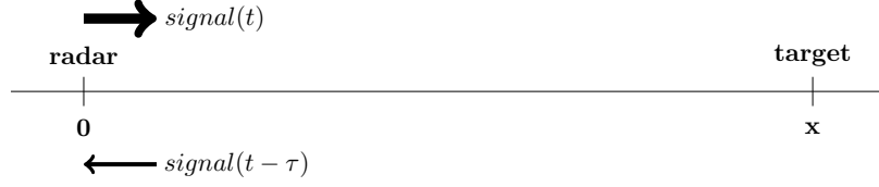
Figure 1.5: The Doppler effect provides an effective way to discriminate between radar targets through the modulation of backscattered pulses due to the movement of targets with respect to the sensor. The phase of the backscattered signal received at time t carries the Doppler information.
