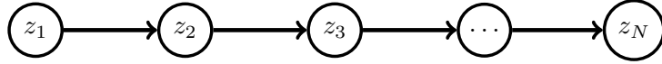
Figure 2.10: Illustration of the close relationship between processing data with a graph neural network and a recurrent neural network. A signal z sampled over N points can be seen as a directed graph with N nodes and N - 1 edges.
