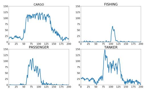
Figure 3.5: Example range profiles (one per class considered). Horizontal axis denotes the range cell index, vertical axis denotes the amplitude.
