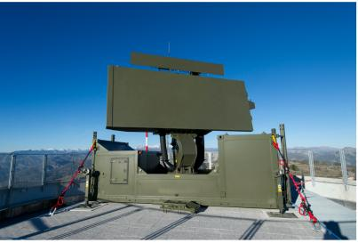
Figure 1.7: The Ground Master air surveillance radars. Notice the rotating antenna, a key factor in the resolution constraints motivating this work. **Top left:** GM 200, medium-range radar **Top right:** GM 60, short-range radar **Bottom:** GM 400, long-range radar. © *Thales*
