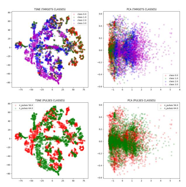
Figure 2.13: 2D visualization of the individual range cell embeddings distribution produced by an FCN as cell2vec, after training. **Top** - each color depicts one target class, i.e. one Doppler pattern. **Bottom** - each color depicts one pulse class, i.e. one Doppler resolution class.
