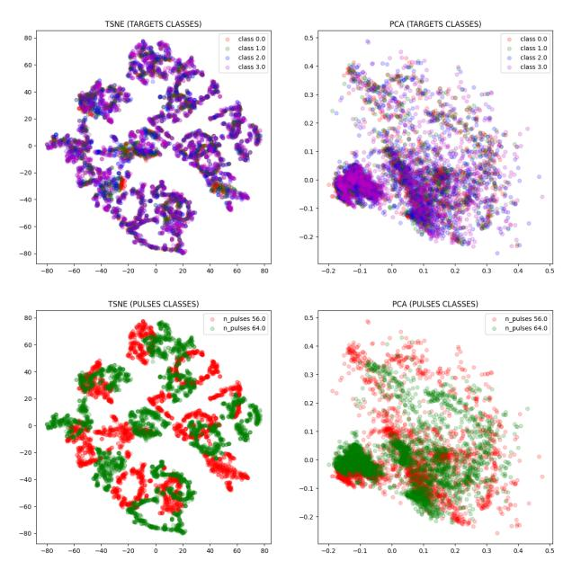
Figure 2.12: 2D visualization of the individual range cell embeddings distribution produced by an FCN as cell2vec, before training. **Top** - each color depicts one target class, i.e. one Doppler pattern. **Bottom** - each color depicts one pulse class, i.e. one Doppler resolution class.
