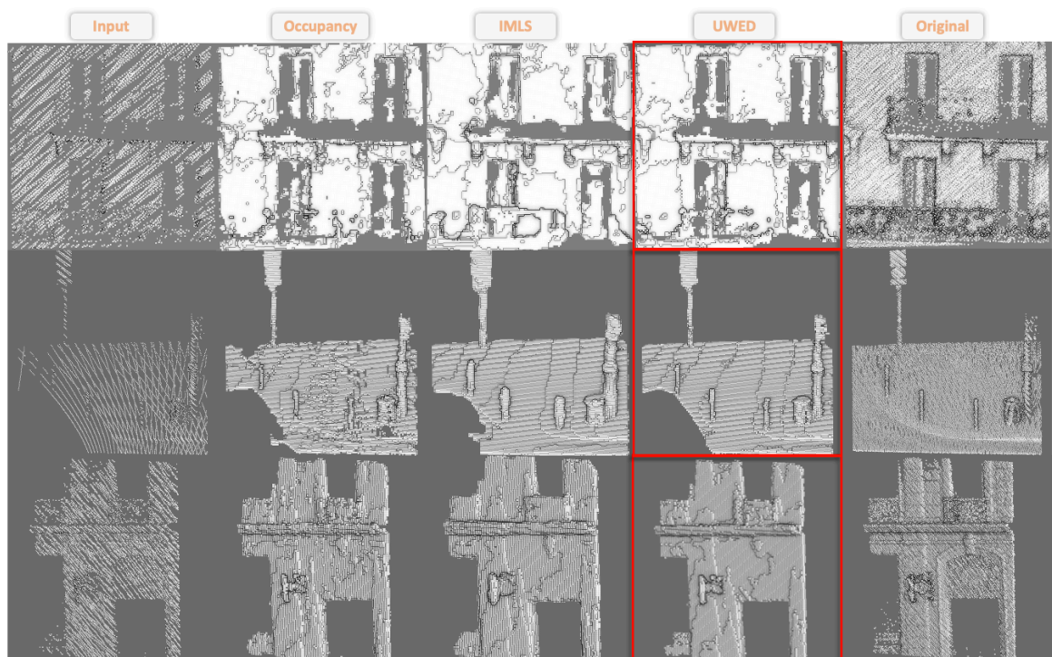
Figure 3.13: Scene completion inference of MinCompNet using Occupancy, IMLS, and our UWED function as input on the PC3D-Paris test set (input has 10% of the original points) and predicting occupancy.
