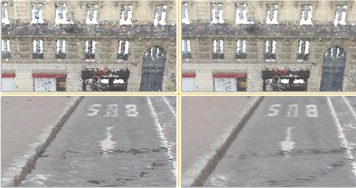
Figure 4.11: Results on rendering the splatted environment with splat-wise color information. We show a rendering of the splatted Soufflot-0 and Soufflot-1 from PC3D-Paris dataset. To the left, we show the rendering without blending. To the right we show the rendering results with blending.
