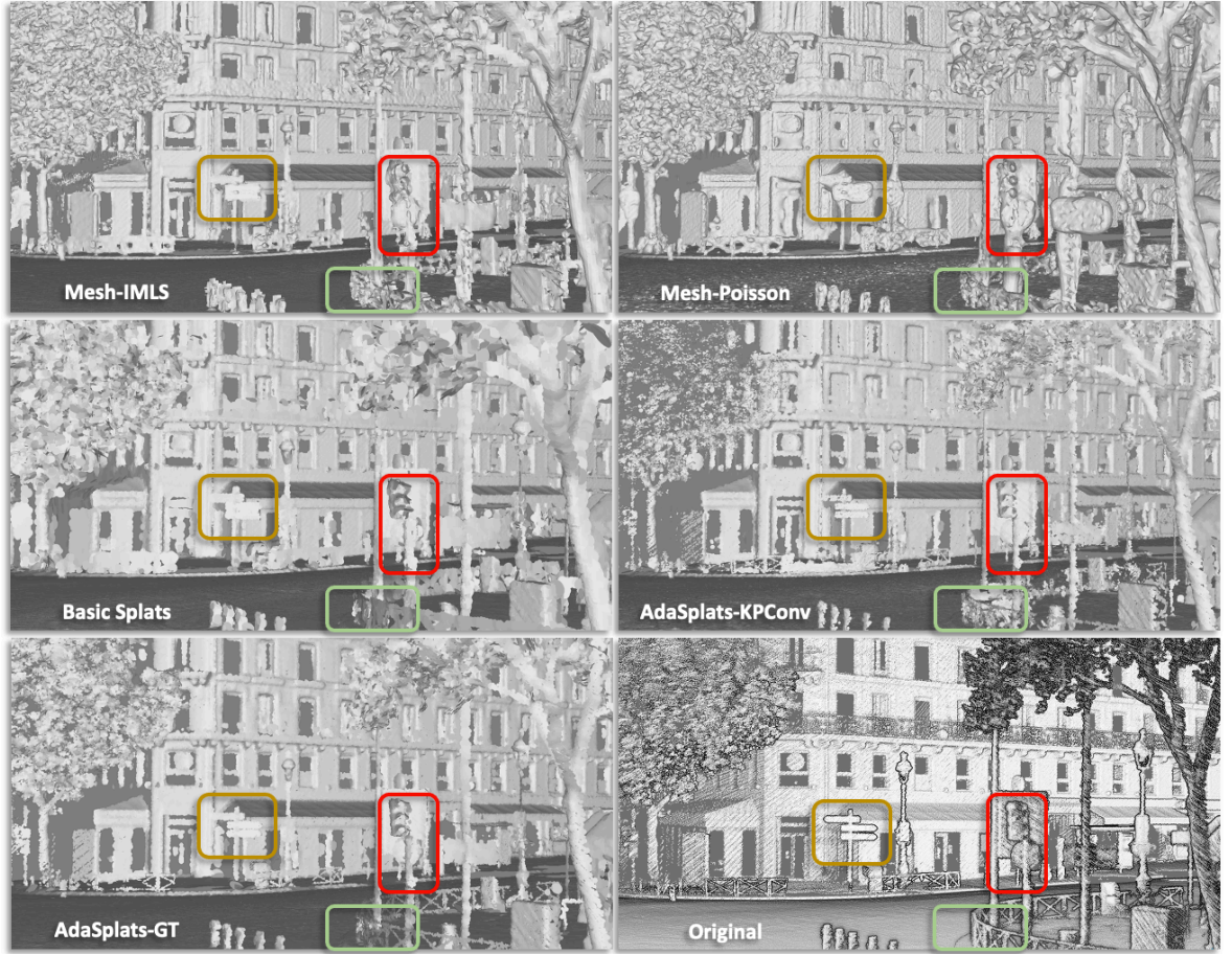
Figure 4.8: Rendering the different surface representations on PC3D-Paris. The first row shows the meshed scene using Poisson (left) and IMLS (right). The second shows the splatted scene using basic splats (left) and AdaSplats using KPConv semantics (right). The splatted scene using AdaSplats-GT, which contains the ground truth point-wise semantic information (left) and the original point cloud (right).
