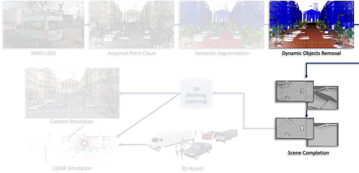
Figure 3.1: The second step in our simulation pipeline consists of removing dynamic objects from the scene and completing missing geometry resulting from object occlusion.
