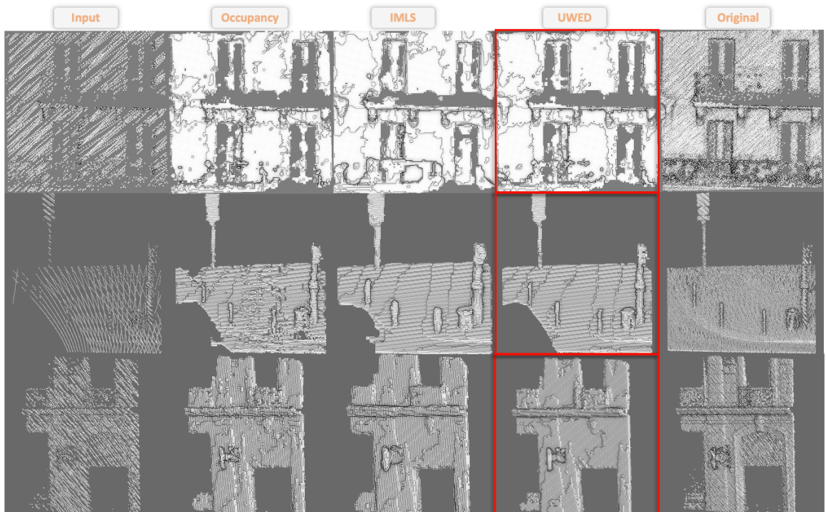
Figure 3.13: Scene completion inference of MinCompNet using Occupancy, IMLS, and our UWED function as input on the PC3D-Paris test set (input has 10% of the original points) and predicting occupancy.
