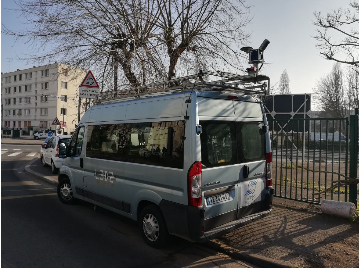
Figure 1.5: The L3D2 Mobile Mapping System of the center of robotics at MINES ParisTech.
