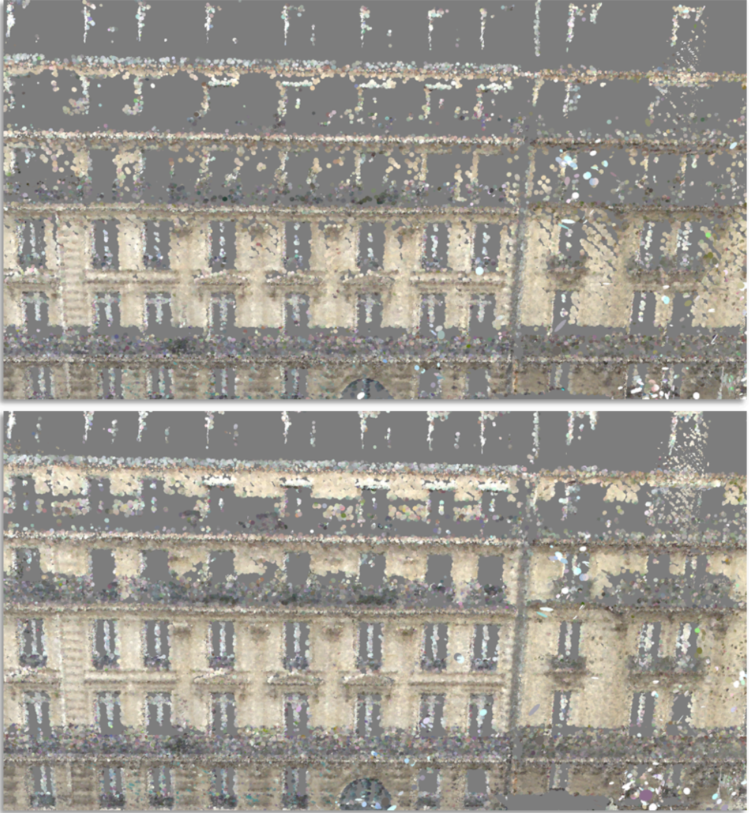
Figure 4.6: Another qualitative evaluation of the resampling algorithm. We show the original and resampled point clouds at the top and bottom, respectively.
