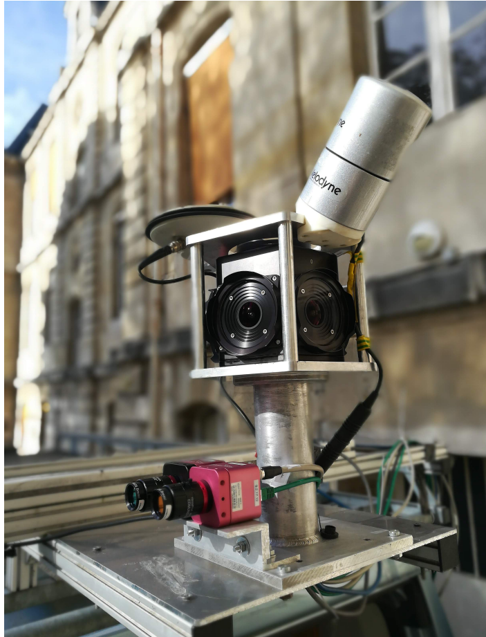
Figure 2.5: Prototype acquisition system used to create the PC3D dataset in the city of Paris. Sensors: Velodyne HDL32 LiDAR, Ladybug5 360° camera, Photonfocus MV1 16-band VIR and 25-band NIR hyperspectral cameras (hyperspectral data is not available in this dataset; they cannot be used in mobile mapping due to a limited exposure time).
