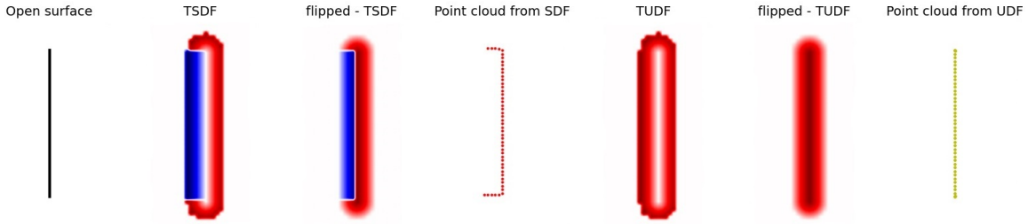
Figure 3.3: A 2D example of an open surface (non-closed surface). Signed distance functions (SDF) do not handle open surfaces, and even if the truncation limits the side effects, the extraction to point clouds will generate border effects. Using an unsigned distance function (UDF), eliminates the problem of negative and positive sides. However, the difficulty lies in the extraction of a point cloud. Here, the point clouds extraction from SDF and UDF follows the methods described in sections 3.3.2.1 and 3.3.2.2 respectively. We also show flipped versions of TSDF and TUDF that remove strong gradients at truncation distance.
