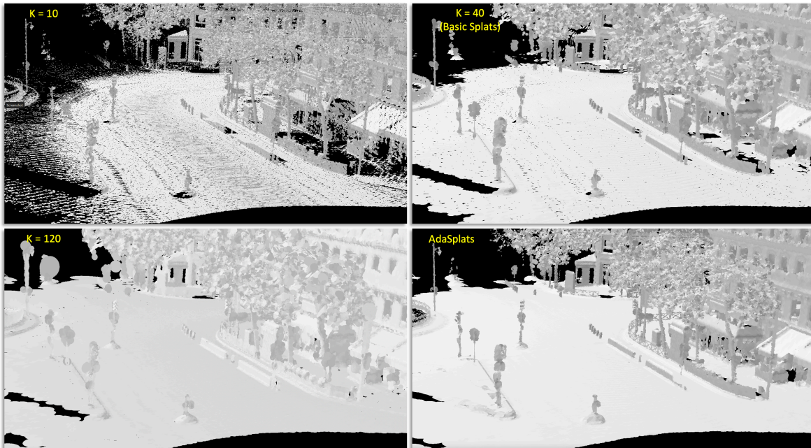
Figure 4.7: Rendering results on different choices of K-nn on PC3D-Paris dataset. A small K (e.g., 10 or 20) results in holes on the surface and ground groups, while resulting in a better approximation on the non-surface and linear groups. A large K (40 to 120) results in a hole-free approximation of the surface and ground semantic groups, while creating artefacts on small structures, belonging to the linear and surface groups.
