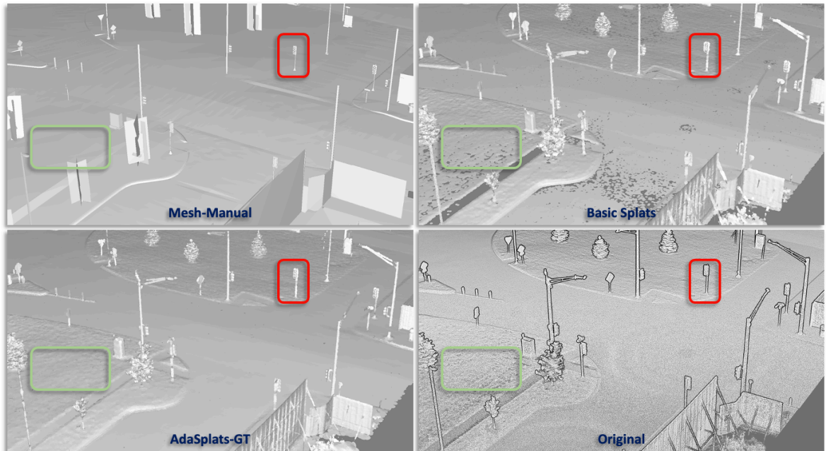
Figure 4.10: Rendering the different surface representations on M-City. The first row shows the manually meshed scene (left) and basic splats (right). The second shows the results of rendering AdaSplats using GT semantics (left) and the original point cloud (right).
