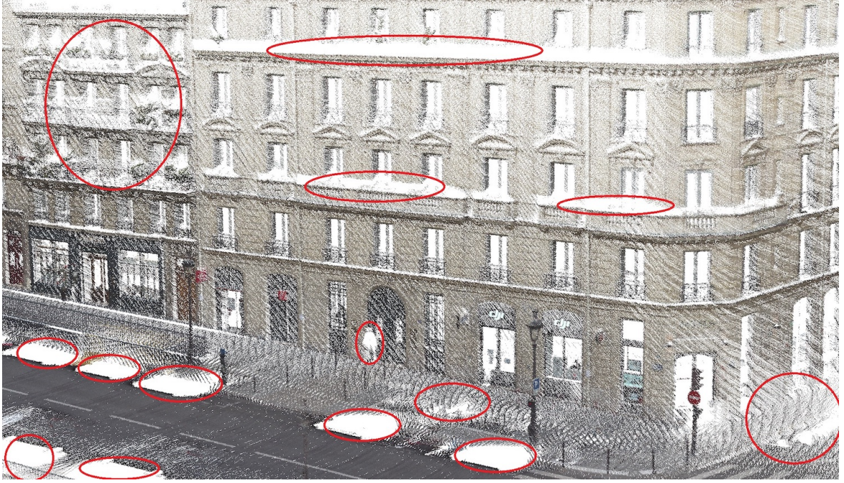
Figure 2.17: Paris data after removal of vehicles and pedestrians. Zones in red circles shows the interest in performing scene completion for 3D mapping: attempt to fill holes from removed pedestrians, parked cars, and to improve sampling of points in areas far from the LiDAR.
