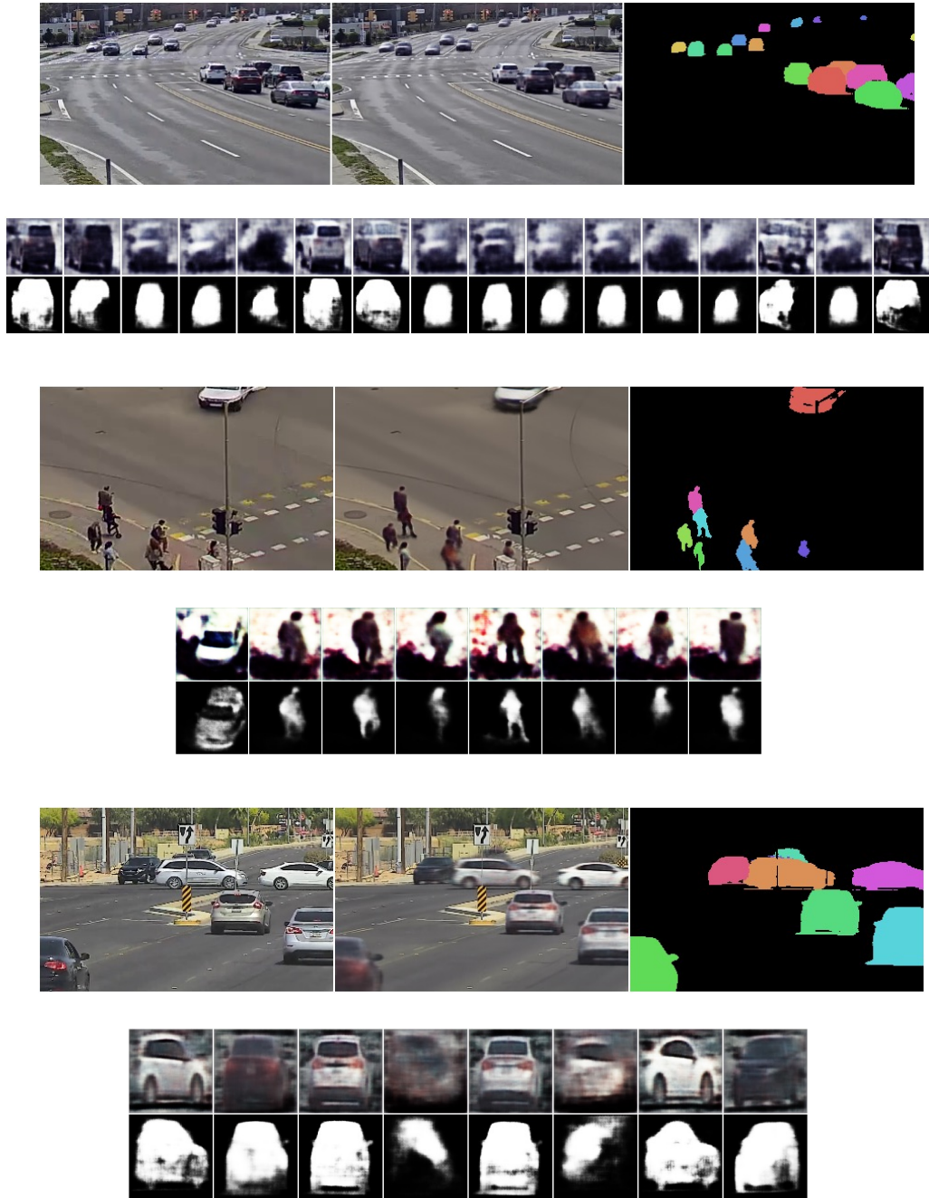
Figure 5.8: Examples of object glimpses generated from real-world traffic videos and associated input images, reconstructed images and predicted segmentation maps
