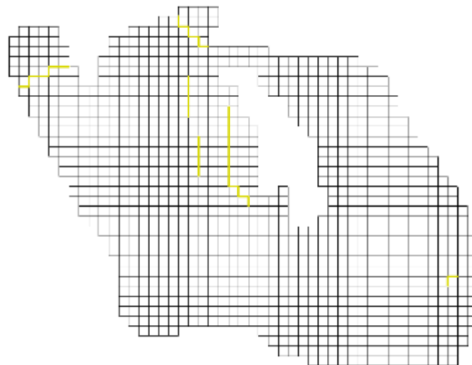
Figure 3.23 – Mathematical mesh used in Delft3D simulation for Lake Champs-sur-Marne. Yellow lines are thin dams
