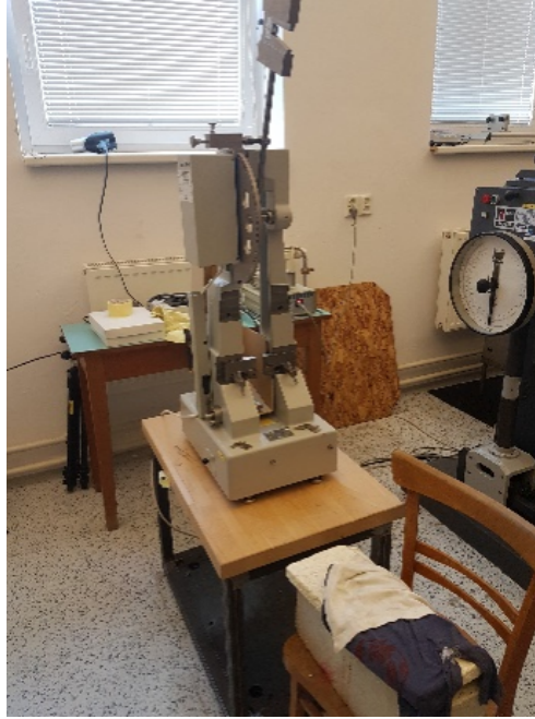
FIGURE 3.25 – Le mouton pendule de Charpy-Zwick 50J (Institute of Physics of Materials, Academy of Sciences of the Czech, Brno)
