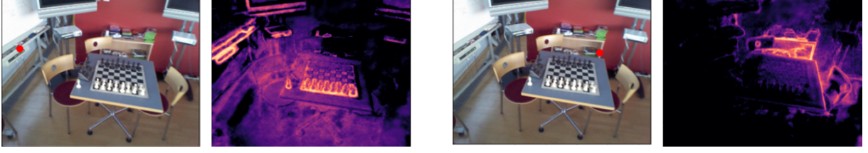
Figure 7.3: Similarities of positional features. We show the dense matching map between one descriptor from the query image (red dots in left images) and the reference descriptors from the neural renderer. Thanks to our training objective, descriptors close (in 3D) to the selected points have high similarity whereas others do not match. This behaviour is enforced by our loss function.
