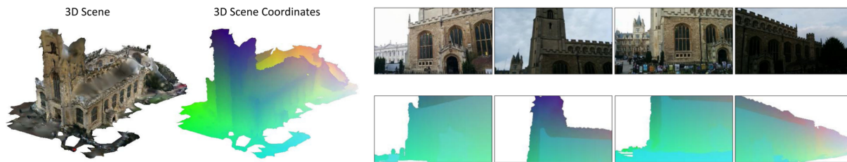
Figure 2.6: Scene Coordinates Regression. 3D scenes coordinates are extracted from a 3D model (left). SCR regresses the 3D coordinates of the visual content observable in the query image (right).
