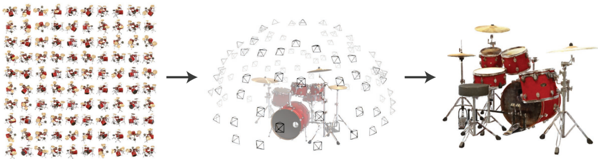
Figure 4.2: Novel view synthesis. Given a sparse set of observations of a scene (left) and their corresponding camera poses (middle), novel view synthesis algorithms are asked to render images of the same scene from unobserved camera poses (right). Figure from [Mildenhall et al., 2020].
