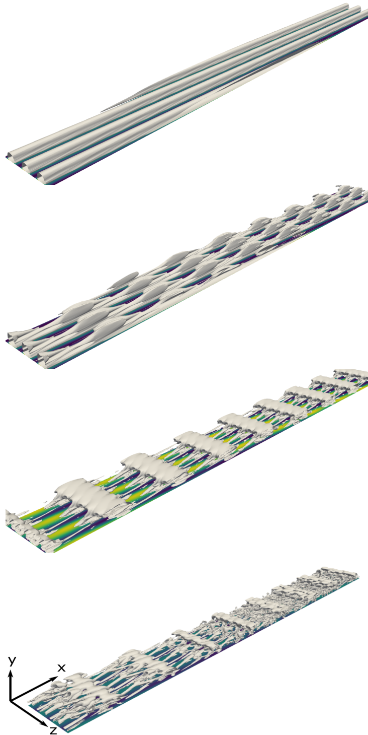
Figure 4.17: Snapshots of the flow at T = 900 , T = 1000 , T = 1050 , T = 1060 , and T = 1080 (from top to bottom). Isosurfaces of the \lambda_2 -criterion, \lambda_2 = -10^{-5} , -10^{-4} , 0.25 , respectively, and contours of the streamwise velocity at the wall. The flow is from bottom to top, and left to right. For the sake of clarity, only half the channel is shown.
