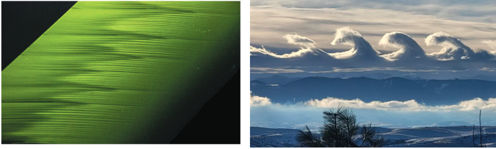
Figure 1.2: Examples of flow patterns resulting from primary instabilities. Left: cross-flow vortices in the transition over a swept plate. Flow is from left to right and darker shades indicate the presence of turbulence. From Serpieri & Kotsonis (2016). Right: Clouds acting as a tracer of Kelvin-Helmholtz waves.
