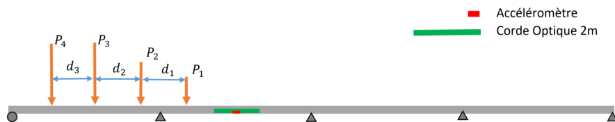
FIGURE 6.1 – Poutre continue soumise aux forces mobiles
