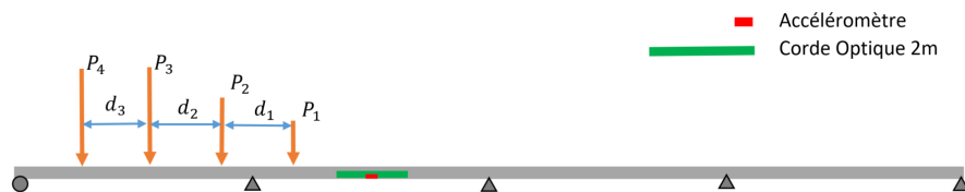
FIGURE 6.1 – Poutre continue soumise aux forces mobiles
