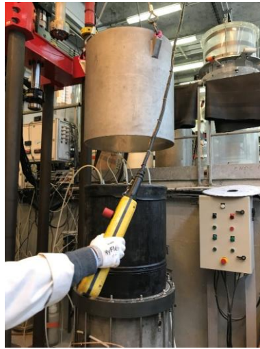
l – setting up the lateral confining cell
