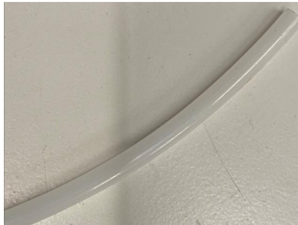
Fig. C-1: Regular pressure loss – flexible connection tube of 4 mm in internal diameter used in the radial injection cell setup.
