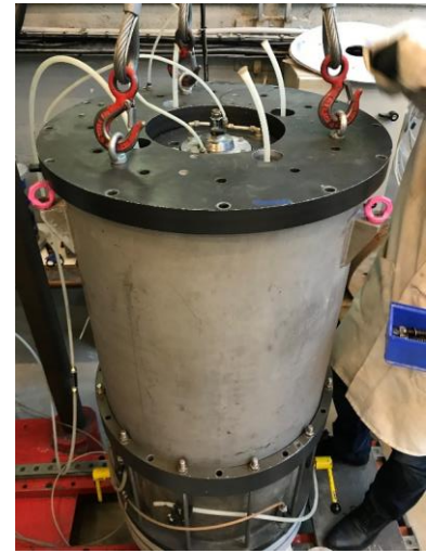
m – installation of the cell cover
