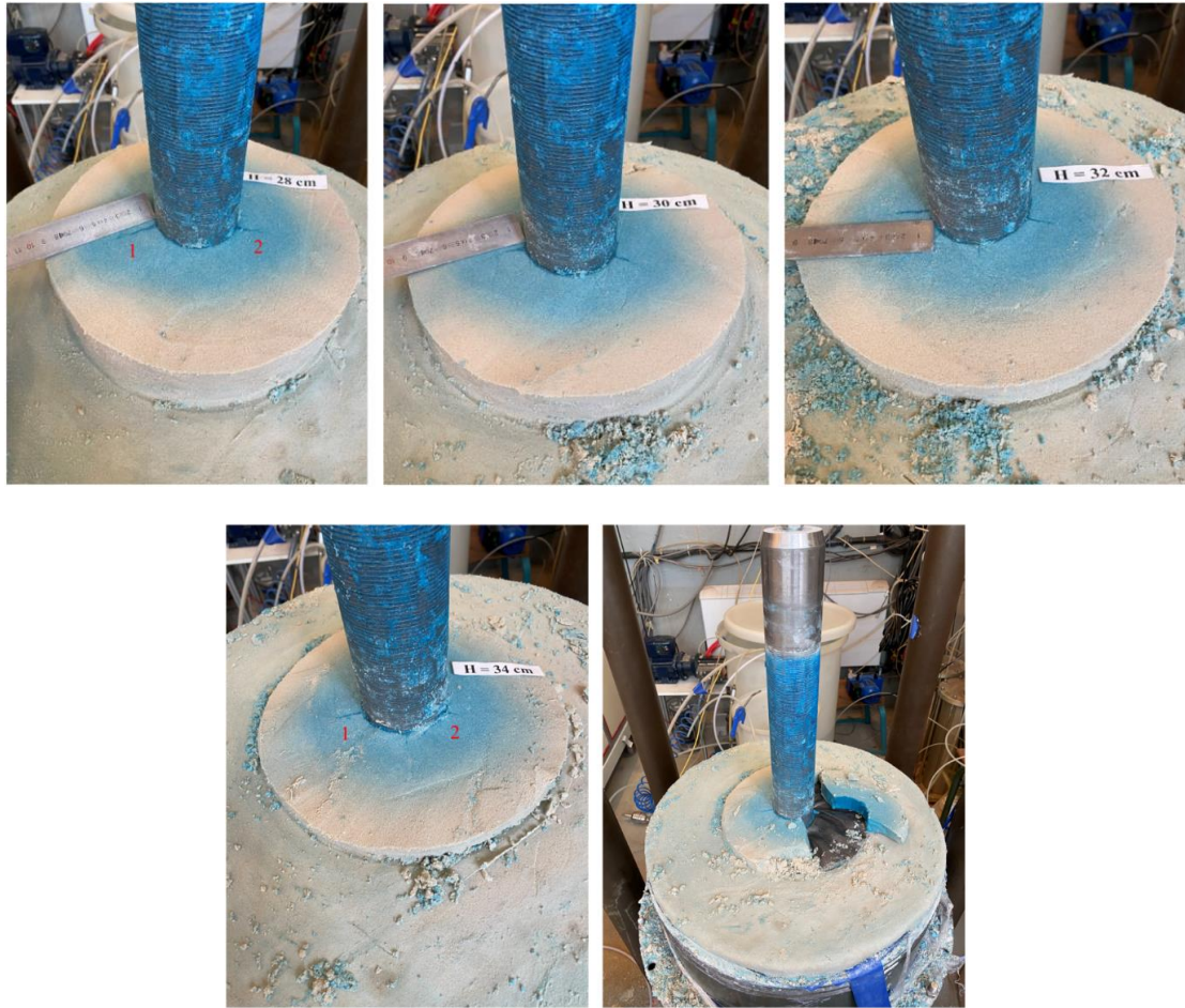
Fig. E-36: Sand pack N34 - Transversal cross-sections of the inner ring at different heights (photos taken by smartphone) (sand pack N32).
