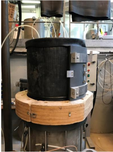
k – applying a vacuum in the sand pack and unmolding
