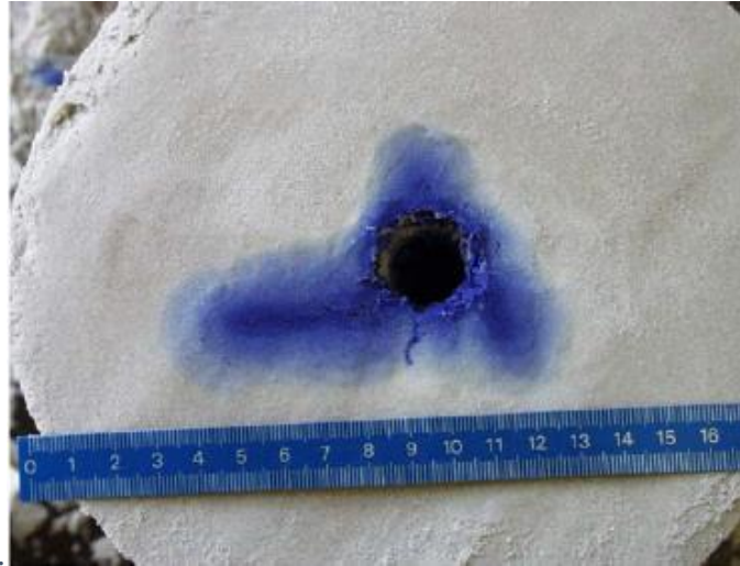
Figure 1.19: Fractures observed while injecting the mixture of borate cross-linked gel and quartz particles ( \sigma_3 = 20 MPa; \sigma_1 = 28.5 MPa; P_{inj\ max} = 55.5 MPa) (Bohloli and de Pater, 2006).
