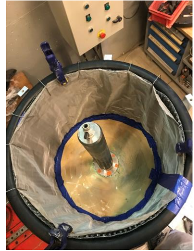
c – installation of the lateral drainage system
