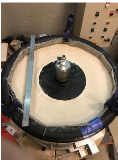
g – setting up a small latex membrane
