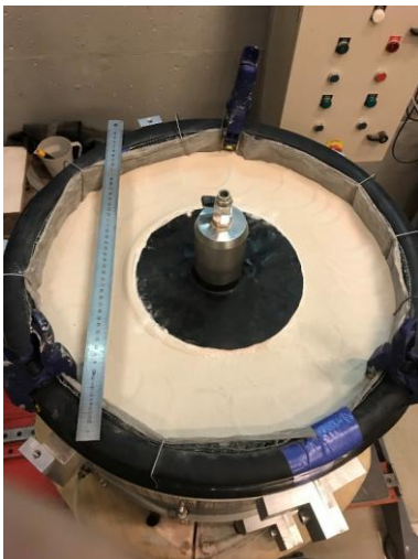
g – setting up a small latex membrane
