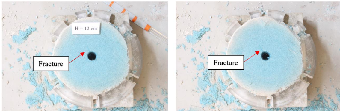
Fig. D-15: Some typical photos of the specimen during excavating (Test P5).
