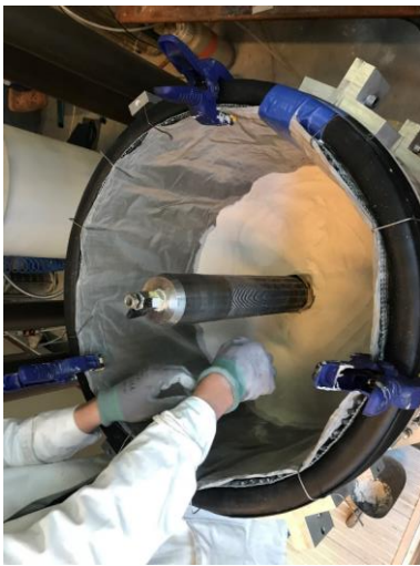
d – compaction of the first low permeability layer
