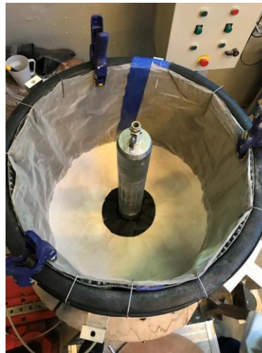
e – setting up a small latex membrane
