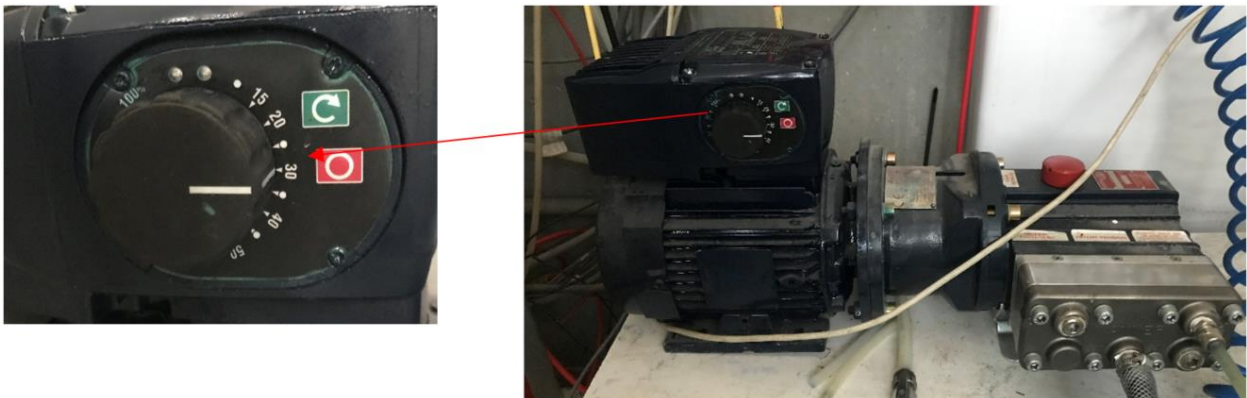
Fig. E-8: Flow control valve of the Wanner Hydra Cell G03 pump.
