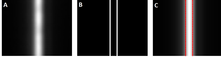
Figure 4.7: Edge detection of a micrometer's line. (A) initial image. (B) detected edges obtained from the vertically averaged image. (C) detected edges displayed (in red) on the initial image of the line.
