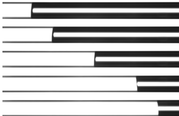
Figure 3.11: Images of an advancing water/air interface acquired by the JAI Spark camera at different instants, for a generated flow rate of 50 nL/min. The dark side is the part with air.
