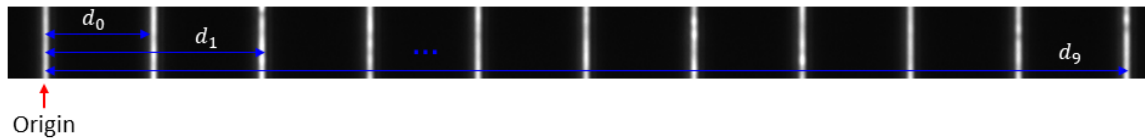
Figure 4.5: Distances measured between the lines of the micrometer to determine the pixel size
