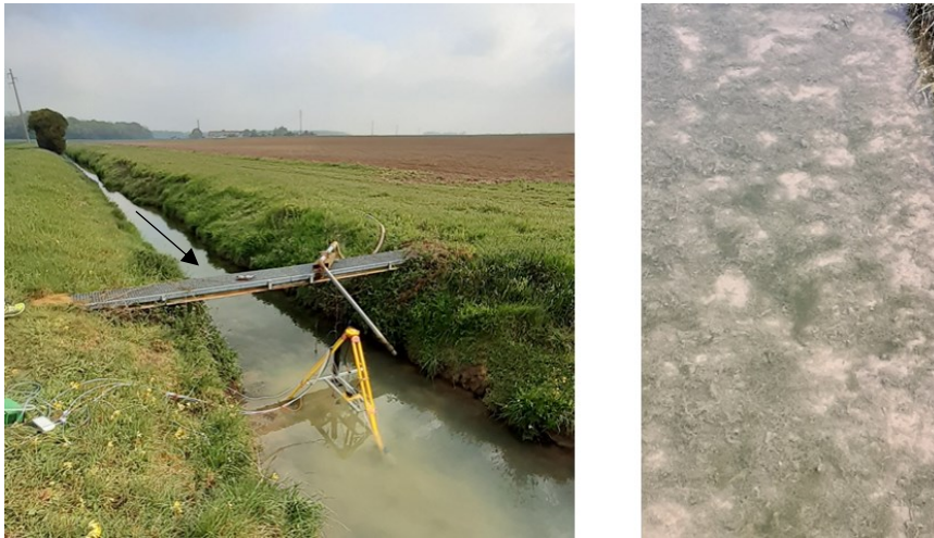
Figure 63 - In the left-hand side the REA and EC placed in the Loge stream. The black arrow denotes the stream flow direction. Water turbidity in the left-hand side photo was the result of prototype deployment. Turbidity was very low during the measurements. On the right, macrophytes and algae in detail on the sediment upstream of the measurement point.
