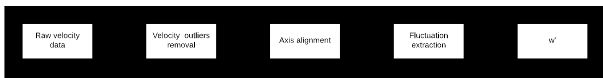
Figure 27 - Velocity processing steps to obtain the fluctuation of the vertical velocity.
