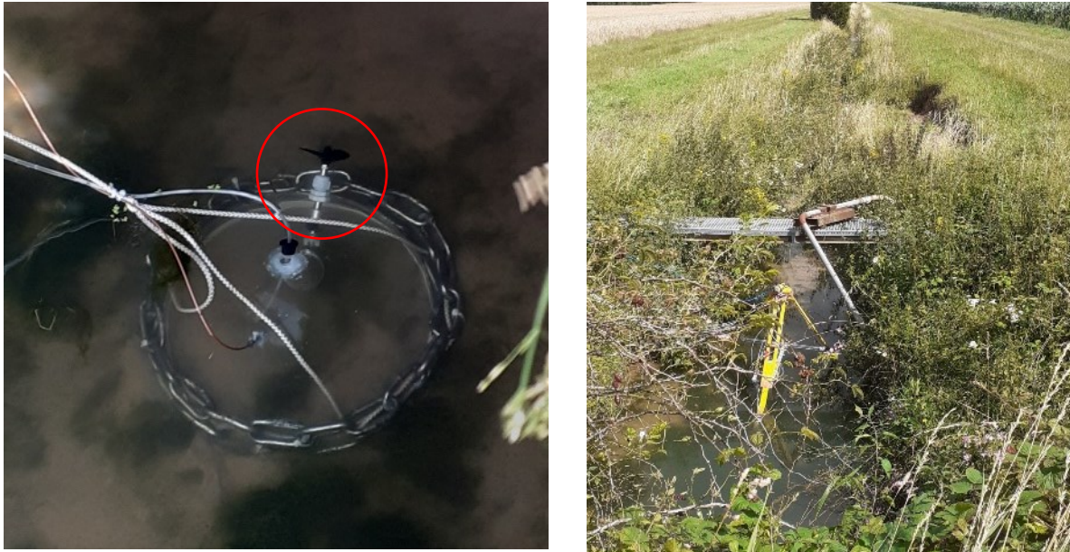
Figure 67 - On the left-hand side of the figure the benthic chamber deployed in the Loge stream. The mixing system is presented by red circle. On the right-hand side, upstream the benthic chamber, REA was deployed. Upstream REA measurement point the stream was no longer straight.
