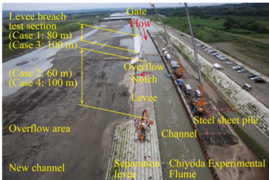
Figure 1.12: Chiyoda experimental flume (Tobita et al. (2014)).
