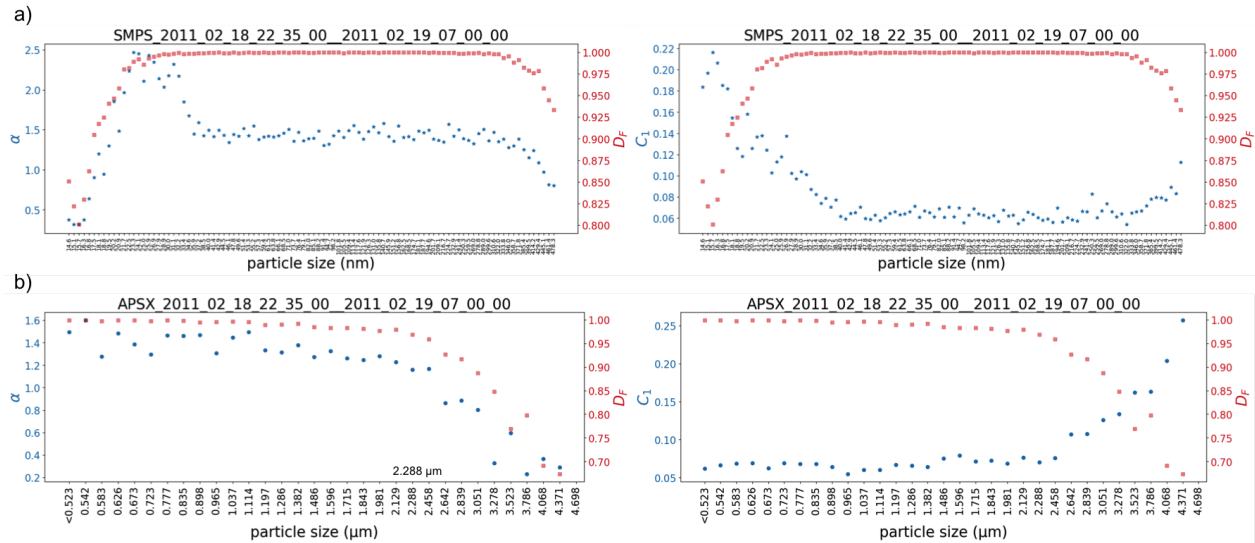
Figure 3.32: Variation of \alpha and C_1 for a) for particles in nm range (SMPS), b) same information for particles in \mu\text{m} range (APS)
