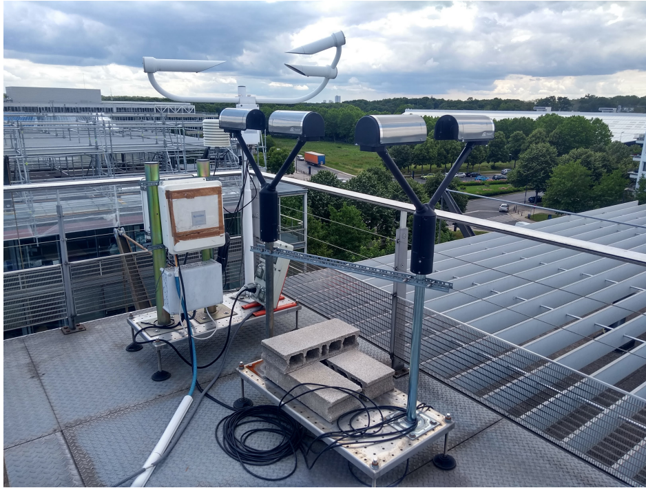
Figure 1.3: Disdrometers devices on TARANIS observatory ( https://hmco.enpc.fr/portfolio-archive/taranis-observatory/ ); two OTT Parsivel 2 devices can be seen on the same base arranged perpendicular to each other, PWS 100 is in the background (in white colour) and can be identified by its receptors positioned at different angles to transmitter (pictures: © Jerry Jose).
