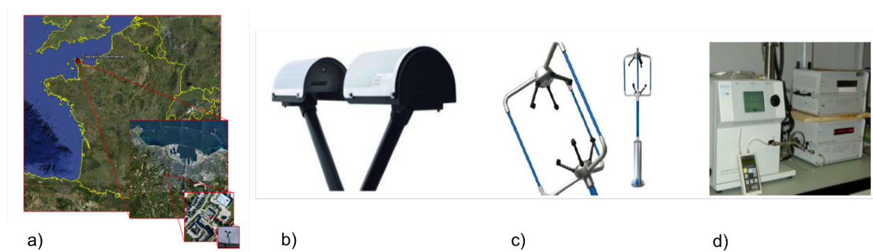
Figure 1.9: a) Location of measurement campaign, b) disdrometer, c) Sonic anemometer and d) Scanning Mobility Particle Sizer (SMPS); images from (Laguionie et al., 2011)
