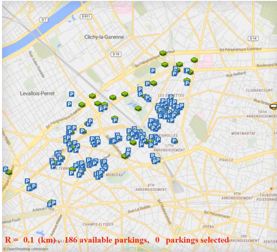
Figure 35. Available delivery spaces result from SPARQL query ( r=100m ) from the semantic environment as the input of AnyLogic.
