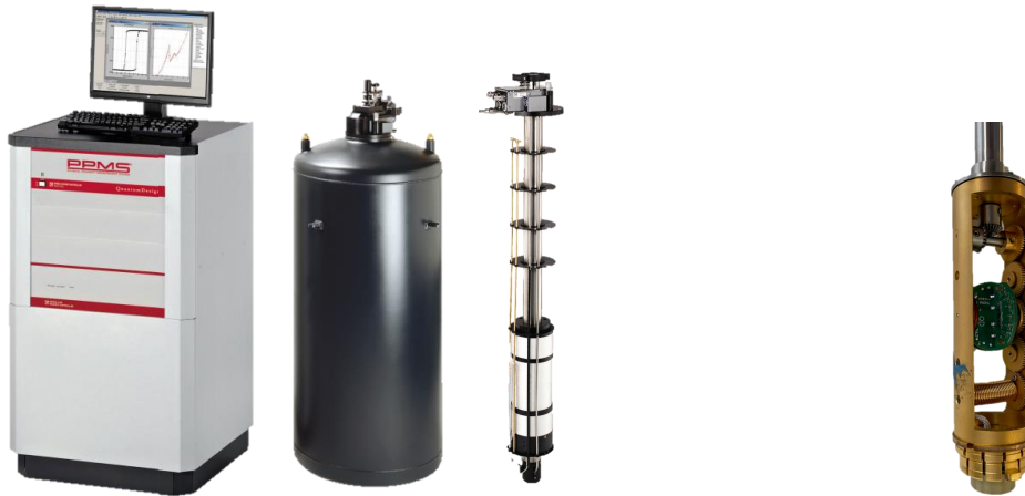
Figure 2.2: Physical Properties Measurement System From left to right : Monitor, ^4\text{He} refrigerator, probe and sample holder for in-plane angle-dependant field measurement.
