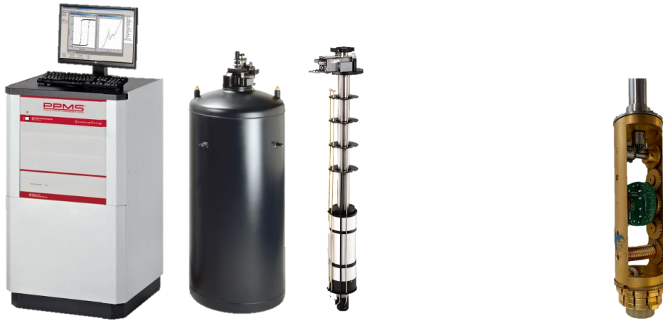
Figure 2.2: Physical Properties Measurement System From left to right : Monitor, ^4\text{He} refrigerator, probe and sample holder for in-plane angle-dependant field measurement.
