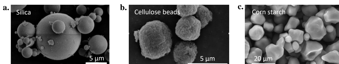
Fig. 6.31 – SEM images from L'Oréal of a. Porous silica (H51) b. Cellulose beads (USF) c. Corn starch (ST 005).
