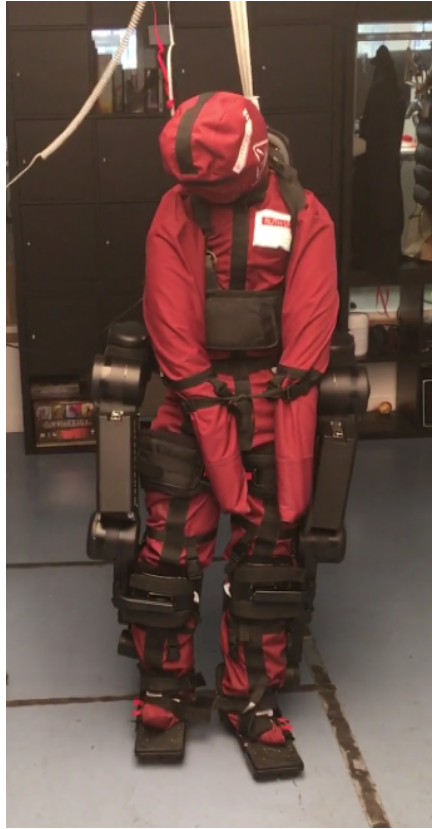
Figure 3.14: Dummy inside Atalante during passive walking (ensures that no user stabilizes the system).
