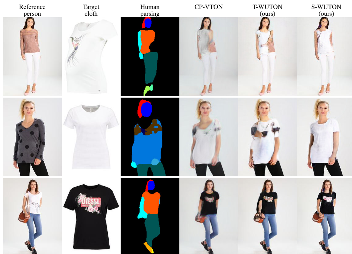
Fig. 4.10 Typical failure cases of the human parser. On the two first rows, it does not segment the person properly. On the third row, it masks the handbag which we would like to preserve in a virtual try-on. CP-VTON and our T-WUTON, which rely on the parsing information, are not robust to a bad parsing. However, the student model S-WUTON which is distilled from the human parser, pose estimator and T-WUTON, can preserve the person’s attributes and does not rely on the parsing information.
