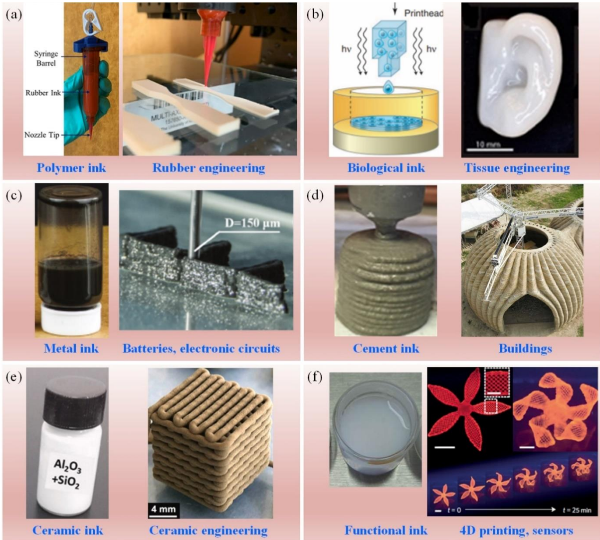
Figure 2.3 Suitable materials and corresponding applications for DIW: (a) polymer ink in rubber engineering[62]; (b) biological ink in tissue engineering[63];(c) metal ink in batteries[64], electronic circuits[65]; (d) cement ink in buildings[66];(e) ceramic ink in ceramic engineering[67]; (f) functional ink in 4D printing and sensors [68]
