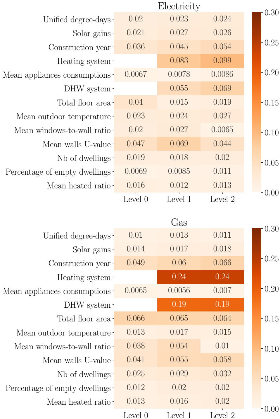
Figure 5.31: Mutual information between the residual obtained with Calomel and buildings characteristics for three levels of data availability
