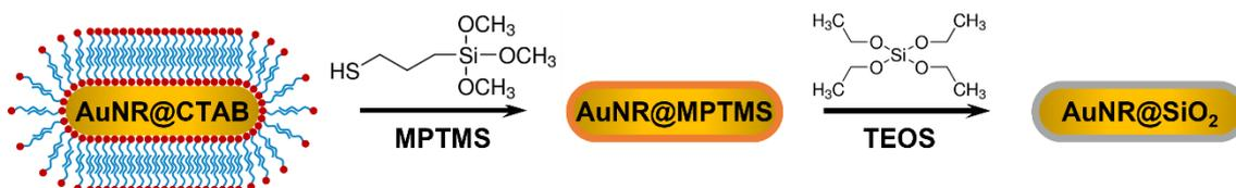
Figure.III.7. Illustration of synthesis of AuNR@SiO<sub>2</sub> core-shell nanoparticles.
