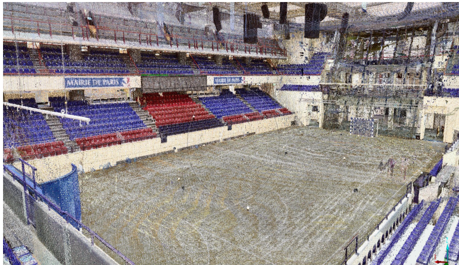
Fig. 4.4 Cloud points of 3-D scan in the grand hall.
