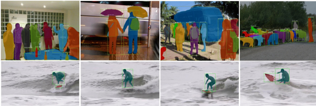
Figure 2.2: The figure shows an example of the instance segmentation for images and videos. The first row displays the instance segmentation task for single RGB images, images from [93]. The second row shows the desired output for video instance segmentation task, images from [284].
