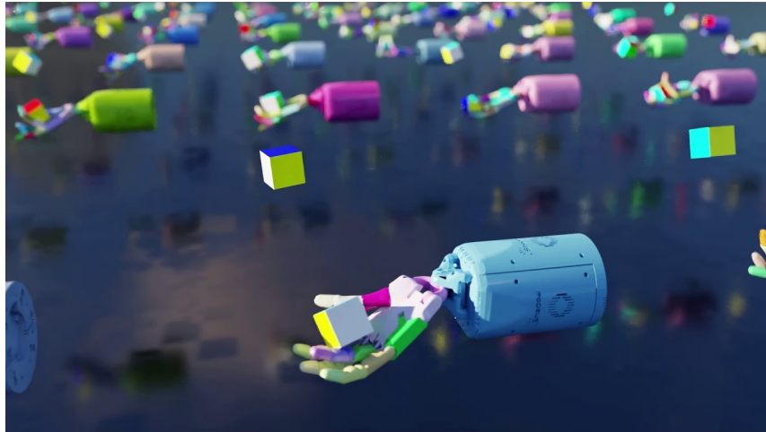
Figure 2.4: The figure shows an example of the grasp simulation in NVIDIA’s Isaac Gym environment, image from [175].
