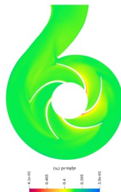
Figure 5.11: Effect of different interphase forces on the volume fraction field of the dispersed phase of the 40%O-60%W emulsion at BEP
