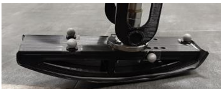
Figure II.27: Pied ROS imprimé en PLA Tough
