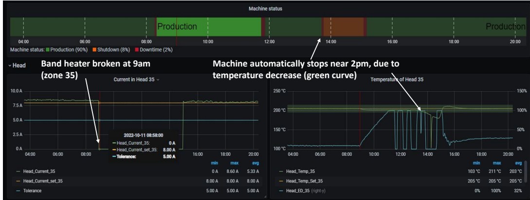
Figure 4.11: Electrical failure of the band heater (Grafana)
