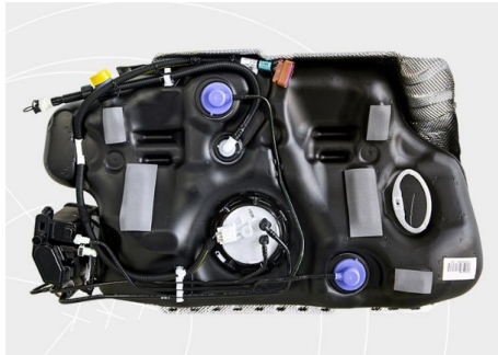
Figure A.2: Plastic fuel tank
