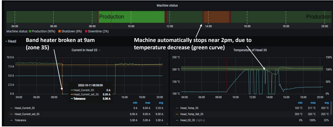
Figure 4.11: Electrical failure of the band heater (Grafana)
