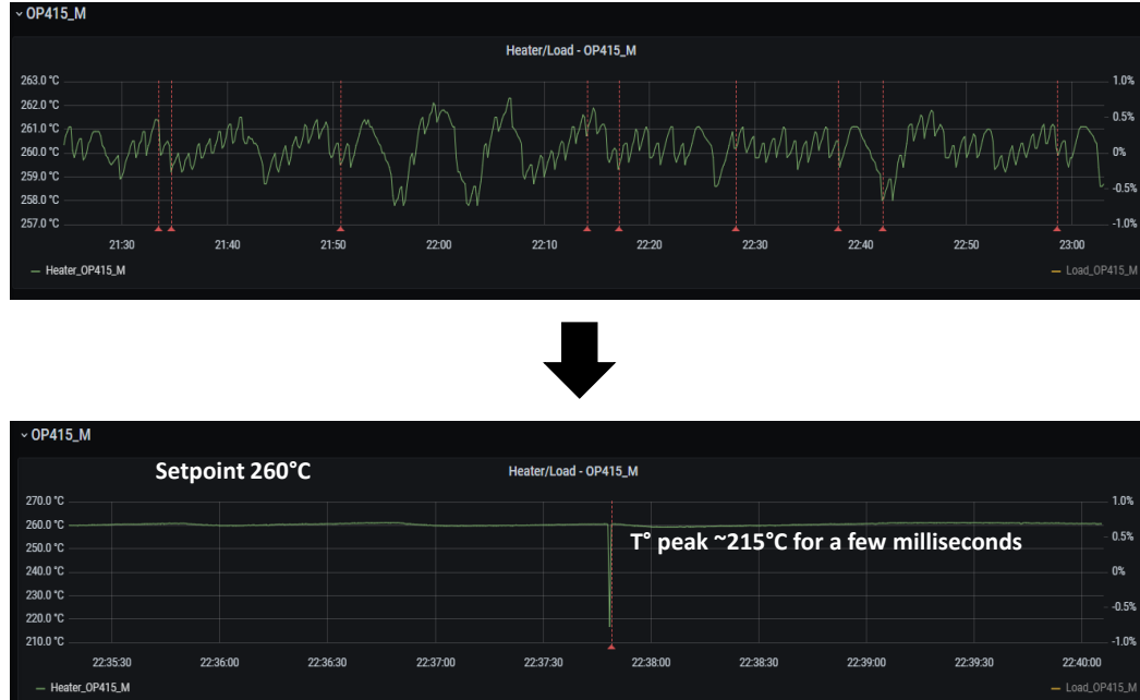
Figure E.1: Detection of failure on thermocouple (Grafana)
