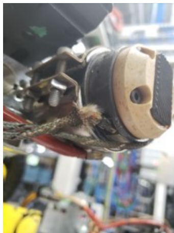
Figure E.2: Thermocouple cable issue
