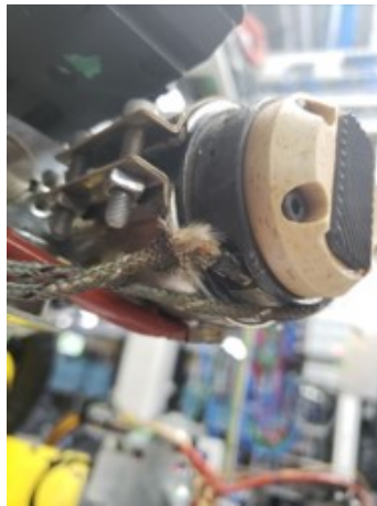
Figure E.2: Thermocouple cable issue
