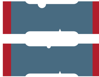
FIGURE 2.31: Two different parameters configurations. Top: R = 7.59 , S = 18.23 , h = 0.84 ; bottom: R = 3.75 , S = 5.58 , h = 1.51 (all dimensions are provided in mm). The red zone is the part subject to rigid body constraints.
